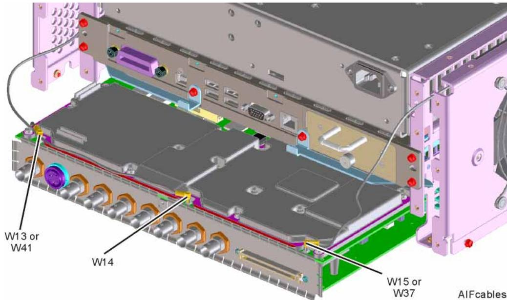
2. Connect the W14 cable to the MMCX female to SMA female adapter. Use an appropriate cable to go from the SMA adapter to the RF input of a functioning spectrum analyzer.
