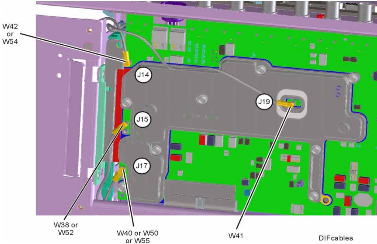
9. Connect the W41 cable to the MMCX female to SMA female connector. Use an appropriate cable to go from the SMA connector to the RF input of a functioning spectrum analyzer to verify the 22.5 MHz I.F. and amplitude is correct.
