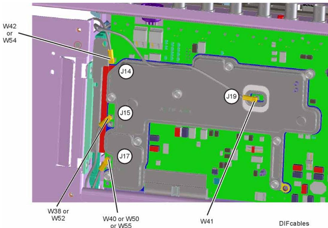
8. Connect the W42 or W54 cable to the MMCX female to SMA female connector. Use an appropriate cable to go from the SMA connector to the RF input of a functioning spectrum analyzer to verify the 100 MHz reference frequency and amplitude is correct.
