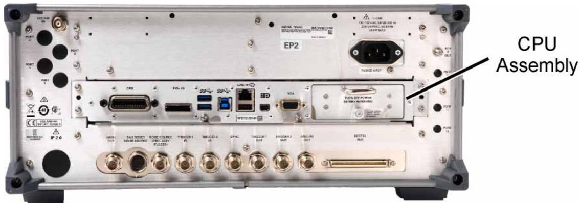
1. Refer to [Figure 15-58](#). Remove the six screws (1) attaching the CPU assembly to the chassis.
