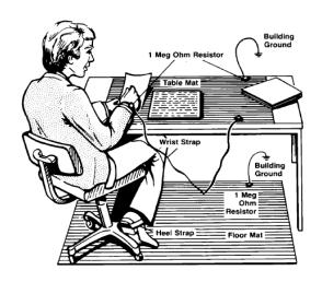
Electrostatic discharge (ESD) can damage or destroy electronic components. Use a static-safe work station to perform all work on electronic assemblies. The figure (left) shows a static-safe work station using two types of ESD protection: conductive tablemat and wrist-strap combination, and conductive floor-mat and heel-strap combination. Both types, when used together, provide a significant level of ESD protection. Of the two, only the table-mat and wrist-strap combination
