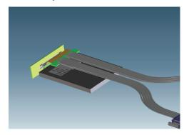
3 Connect the interposer cables to the U4301A/B analyzer module to match your testing requirements.
