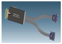
Insert the disk drive with interposer attached, into the drive bay.
