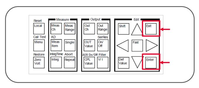
Step 6. Press the Exit key twice to close the setup menu.
