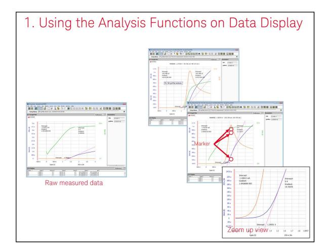
The Auto-analysis and graphical display features of EasyEXPERT help to accelerate your analysis, providing many powerful analysis tools such as auto-scaling, marker and line operation, multiple Y axes capabilities etc. For example, the data display and intuitive GUI operation allows for the quick extraction of the threshold voltage by finding the max position on the gm curve in Y2, drawing the tangent line on the ld curve in Y1 and reading out the intercept to the X axis, as illustrated below.
