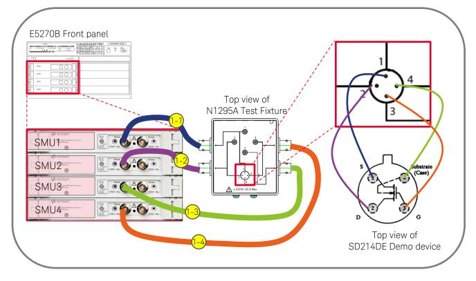
Step 1. Connect the instrument to the Fixture (N1295A)
