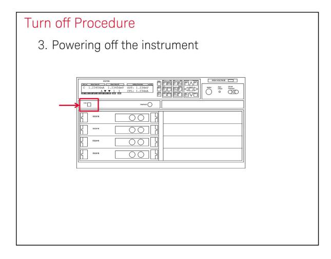
3. Power off the instrument by pressing the "Line" button.
