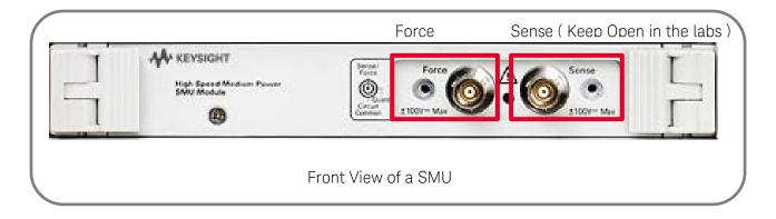
Note: A Sense line is used for high current measurement or low resistance measurement to minimize the measurement error caused by the residual resistance of the connection cables.
