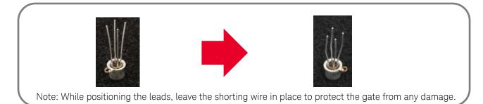
Step 2-2. Insert the device (SD214DE) into the socket on the Test Fixture
