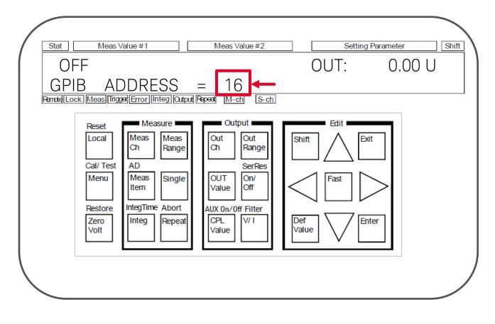
Step 5. Press the Enter key to make the setup effective, or press the Exit key to cancel any changes to the setup.
