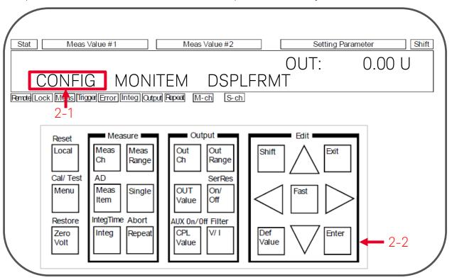
Step 2. Move the cursor to CONFIG, and then press the Enter key.
