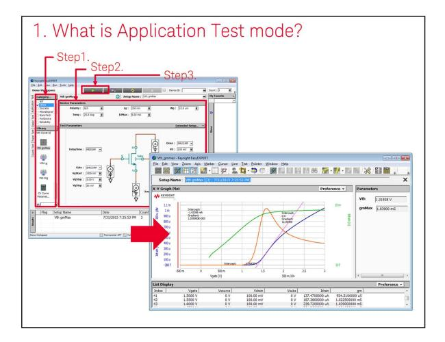
Application Test Mode supports measurements in three easy steps by utilizing extensive libraries of hundreds of pre-defined tests.
