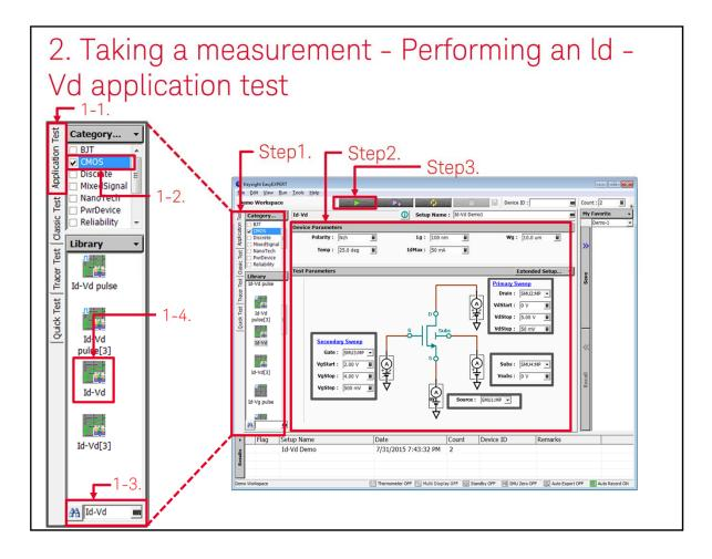
Let's start the Lab. Using application test mode, measurements can be executed in three simple steps.
