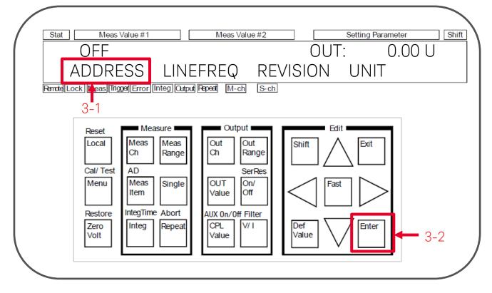
Step 4. Press the arrow keys to set the GPIB address.
