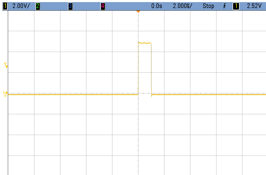
Figure 1-5 Oscilloscope signal pulse at KtM9217A PXIe 2-CH Digitizer external front connector when trigger event is accepted at PXI_TRIG0
