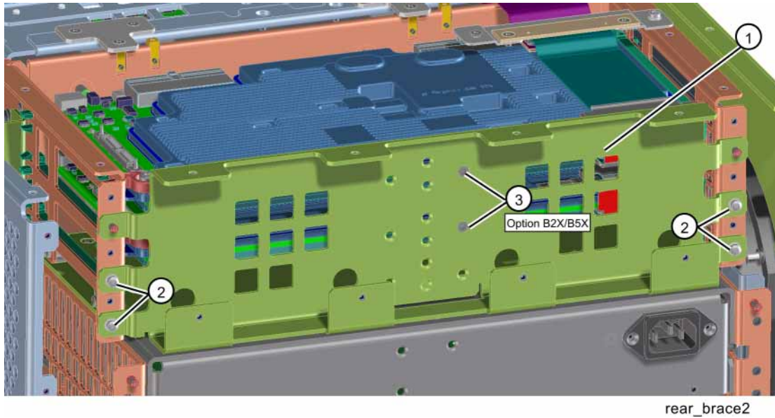
Figure 15-74 Rear Brace Removal Serial Number Prefix \geq 5605 and All Options 544 and 550
