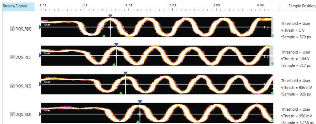
Figure 7. Burst qualified eye scan allows you to view the activity on the signals only when a burst is taking place. The screenshot above shows DDR4 2400 Mb/s read DQS 0-3 scanned in signal trace mode with no back-to-back bursts, allowing the user to view the DDR4 read strobes relative to each other, including the strobe pre-embles.
