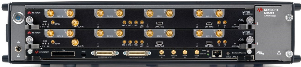
Figure 3. Two M9703B digitizers installed in the M9502A 2-slot chassis, forming a 16-ch 12-bit acquisition system
