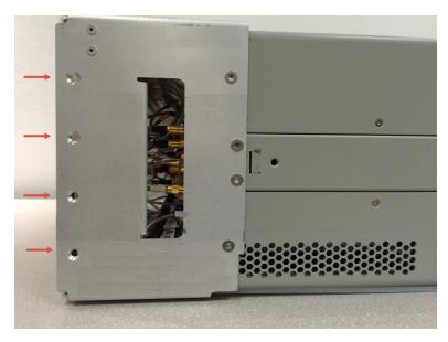
The left and right flanges are indentified with an "L" and an "R" respectively. The following image shows the right side flange attached.
