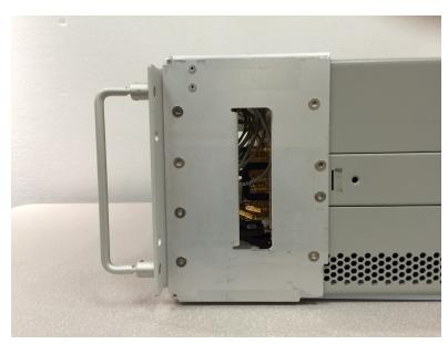
Once both the left and right flanges are attached, the M9018A chassis assembly is ready to be installed in the rack.
