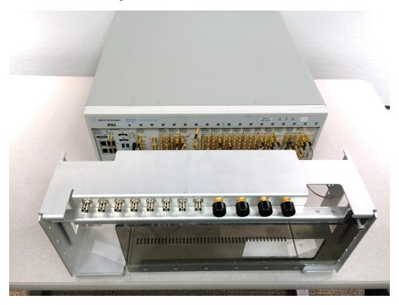
Cables from the connectors on the Y1270A frame are routed and terminated on PXI module connectors in the M9018A chassis.
