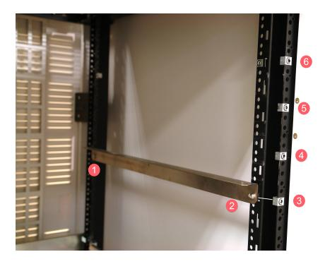
Step 5: Slide the M9018A Chassis into the Rack.
