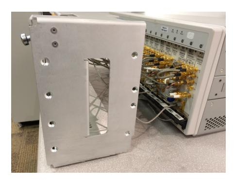
The following is the procedure for mounting a M9018A chassis with an attached Y1270A frame into a standard 19" instrument rack.
