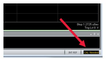
When a calibration is needed, user can either launch it from **Utilities > Calibration** or by clicking on **CAL**: **Needed**.
