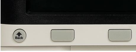
Use the six softkeys (two shown here) to navigate through the menus. Press the round **[Back]** key to return to the previous menu.
