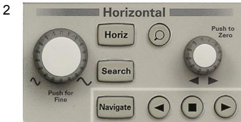
Configure the horizontal axis and navigate through the waveform.
