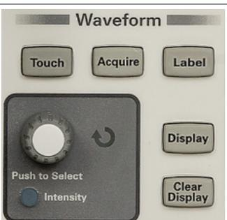
Specify, adjust and annotate the way the waveform is displayed. Enable or disable the touchscreen for enhanced usability.
