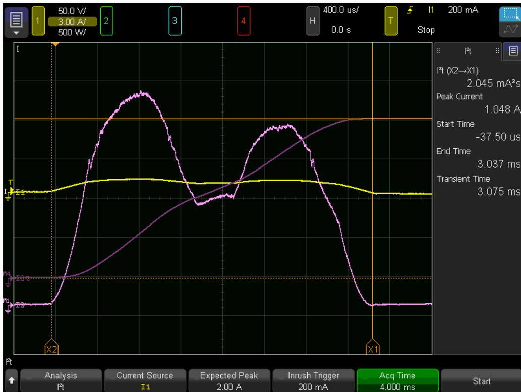
The bright horizontal yellow line is the current signal (I). It is yellow in this case because the Current Source is Channel 1. The bumpy, bright magenta line is a math function, the square of the current (I<sup>2</sup>). The rising purple line is the integral of the I<sup>2</sup> signal over time (I<sup>2</sup>t). The orange vertical and horizontal lines are the cursors delimiting the calculations shown in the sidebar.
