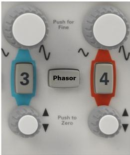
On the PA2201A or the PA2203A, you can press **[Display] > Phasor**, or you can use the blue menu symbol in the upper left corner of the display.
