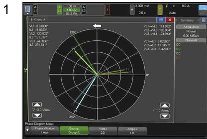
The color display (800x600 pixels) is the heart of the power analyzer's user interface.
