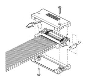
The alternate thumb screw hood consists of six pieces:
