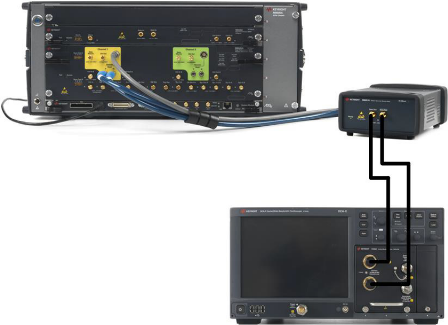
Connection among M8045A, M8057A/B and N1000A with N1060A
