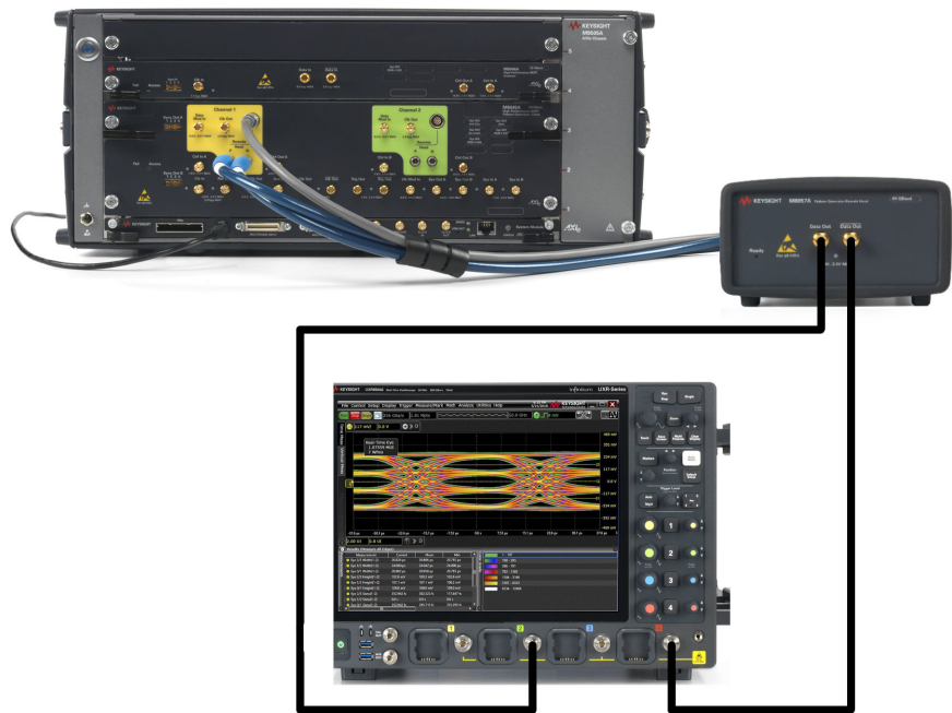
Connection among M8045A, M8057A/B and UXR-series oscilloscope
