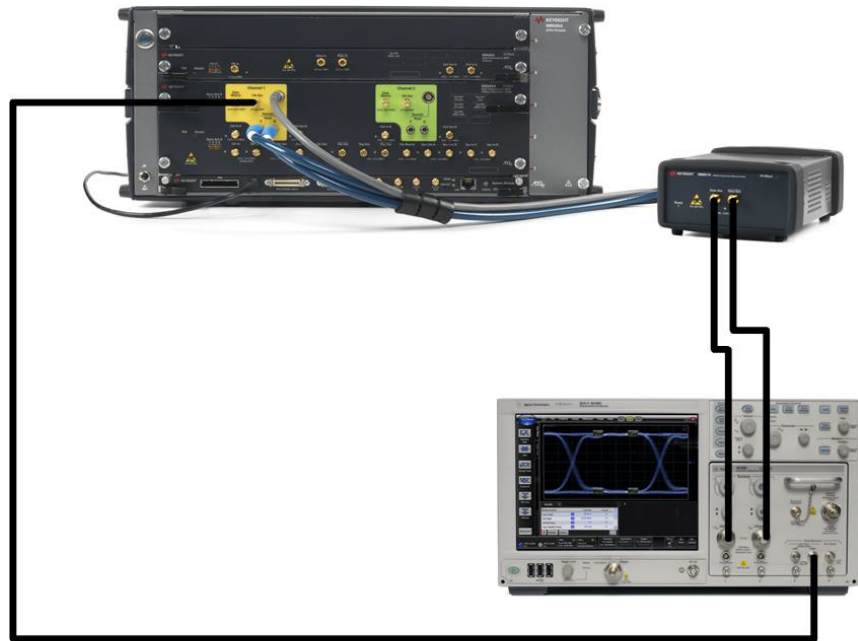
Connection among M8045A, M8057A/B and 86100D with 86108B
