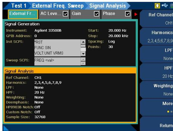
**Figure 7-44** External Frequency Sweep > Signal Analysis settings menu page
