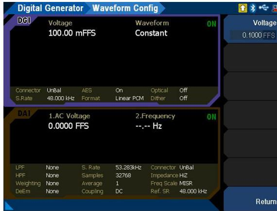
Figure 3-41 Digital Generator > Waveform Config menu page (constant)
