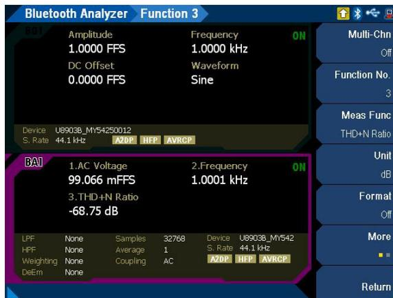
Figure 4-20 Bluetooth Analyzer > Functions > THD+N Ratio menu page 1
