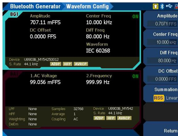
Figure 3-21 Bluetooth Generator > Waveform Config menu page (IEC 60268 waveform)
