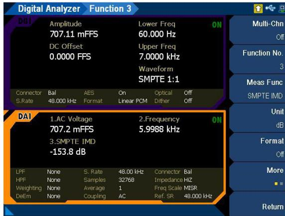
Figure 4-34 Digital Analyzer > Functions > SMPTE IMD menu page 1
