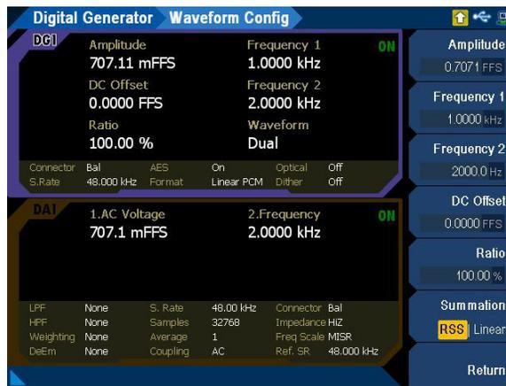
Figure 3-11 Digital Generator > Waveform Config menu page (dual waveform)
