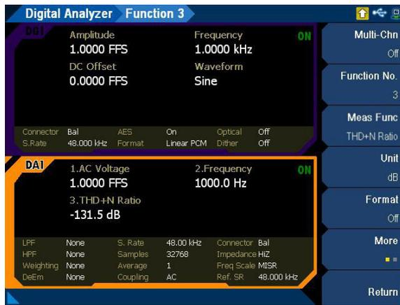
Figure 4-19 Digital Analyzer > Functions > THD+N Ratio menu page 1
