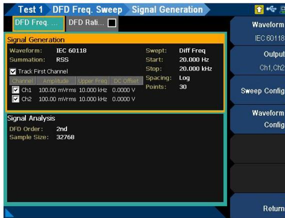
**Figure 7-41** DFD Frequency Sweep > Signal Generation settings menu page
