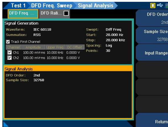
**Figure 7-42** DFD Frequency Sweep > Signal Analysis settings menu page
