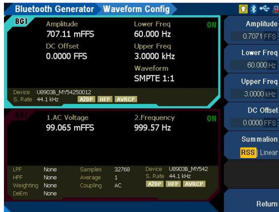
Figure 3-15 Bluetooth Generator > Waveform Config menu page (SMPT 1:1 waveform)
