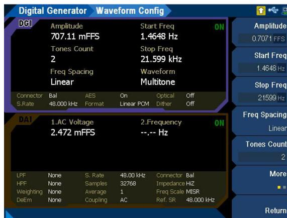
Figure 3-49 Digital Generator > Waveform Config menu page 1 (multitone waveform)
