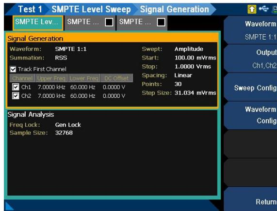
**Figure 7-47** SMPTE Level Sweep > Signal Generation settings menu page
