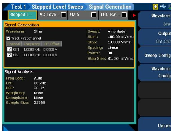
**Figure 7-45** Stepped Level Sweep > Signal Generation settings menu page
