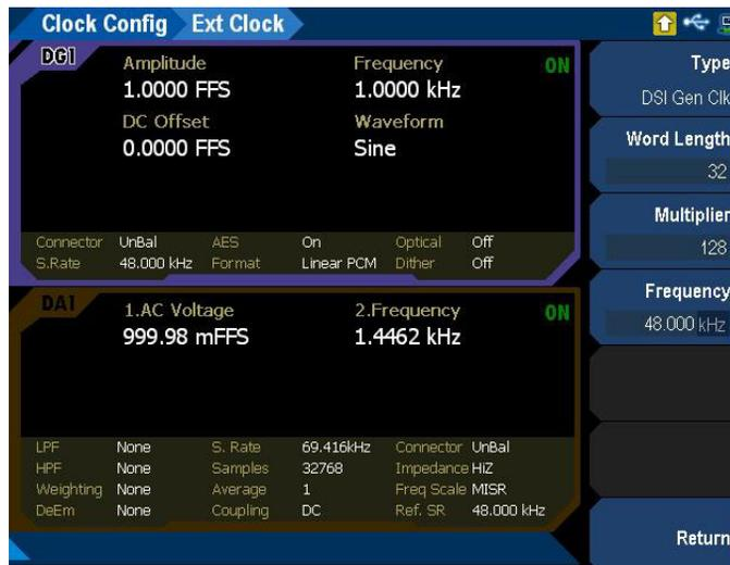
**Figure 3-60** Digital Generator > Clock Config > External Clock menu page
