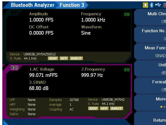
Figure 4-26 Bluetooth Analyzer > Functions > SINAD menu page 1
