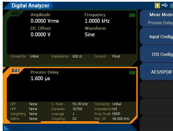
Figure 4-4 Digital Analyzer menu page (process delay measurement mode)
