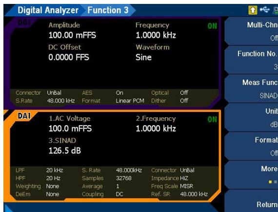
Figure 4-25 Digital Analyzer > Functions > SINAD menu page 1
