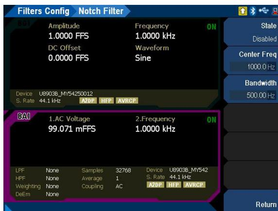
**Figure 4-55** Bluetooth Analyzer > Filter Config > Notch Filter menu page**Table 4-26** Bluetooth Analyzer > Filter Config > Notch Filter menu description
