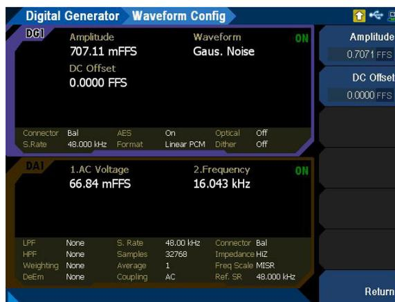
Figure 3-23 Digital Generator > Waveform Config menu page (Gaussian noise)
