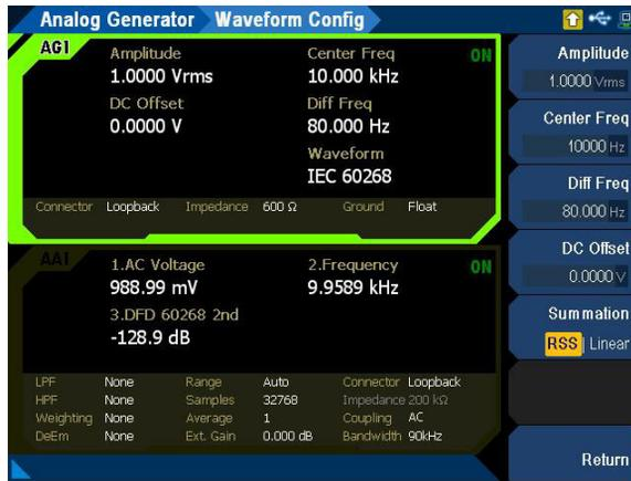
**Figure 3-19** Analog Generator > Waveform Config menu page (IEC 60268 waveform)
