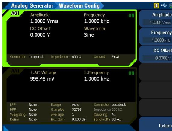
**Figure 3-4** Analog Generator > Waveform Config menu page (sine waveform)
