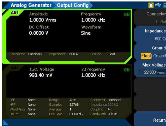
**Figure 3-56** Analog Generator > Output Config menu page
