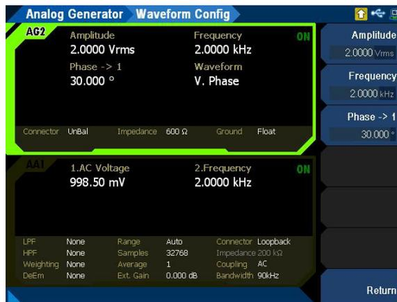
**Figure 3-7** Analog Generator > Waveform Config menu page (variable phase waveform)
