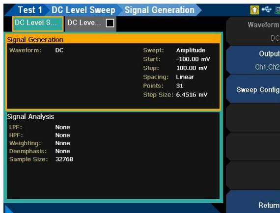
**Figure 7-51** DC Level Sweep > Signal Generation settings menu page
