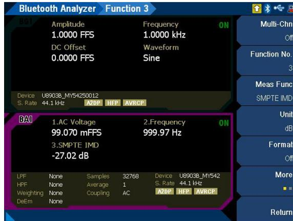
Figure 4-35 Bluetooth Analyzer > Functions > SMPTE IMD menu page 1
