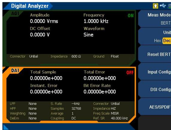
Figure 4-5 Digital Analyzer menu page (BERT measurement mode)
