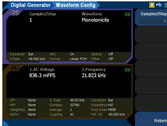
**Figure 3-40** Digital Generator > Waveform Config menu page (monotonicity)
