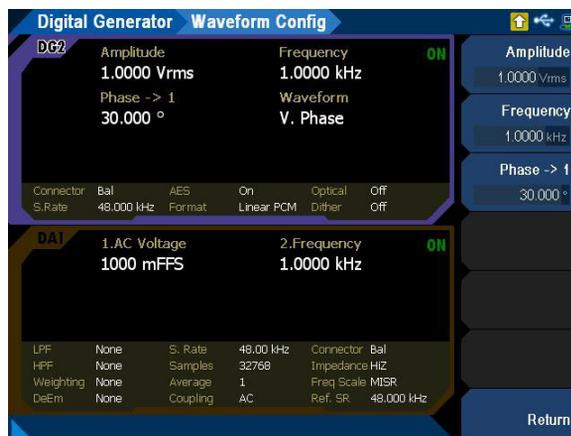
**Figure 3-8** Digital Generator > Waveform Config menu page (variable phase waveform)
