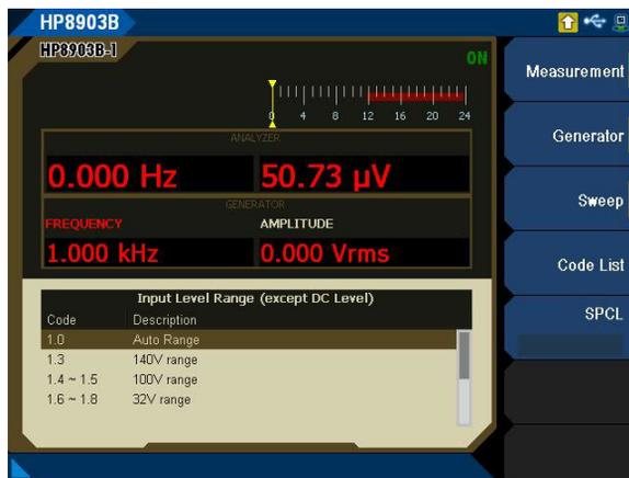
**Figure 8-5** HP8903B > Code List menu page (Input Level Range (except DC Level))
