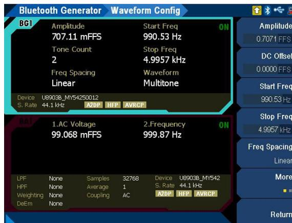
Figure 3-50 Bluetooth Generator > Waveform Config menu page 1 (multitone waveform)
