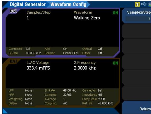
**Figure 3-43** Digital Generator > Waveform Config menu page (walking zero)
