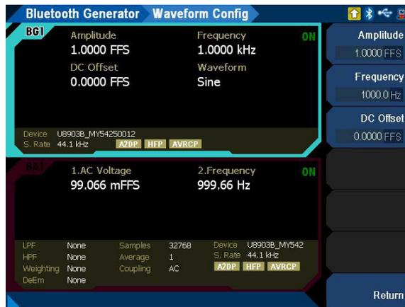
Figure 3-6 Bluetooth Generator > Waveform Config menu page (sine waveform)
