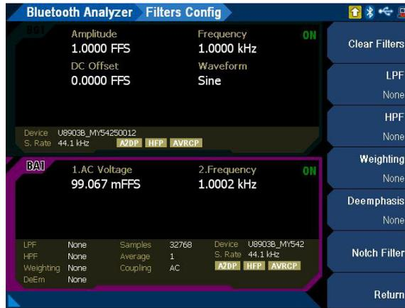
**Figure 4-54** *Bluetooth Analyzer* > Filter Config menu page
