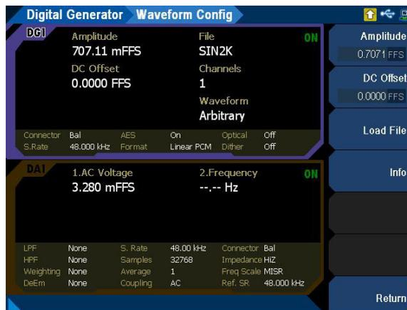
Figure 3-46 Digital Generator > Waveform Config menu page (arbitrary waveform)
