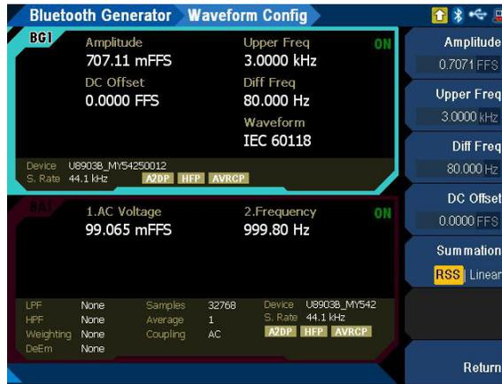
Figure 3-18 Bluetooth Generator > Waveform Config menu page (IEC 60118 waveform)
