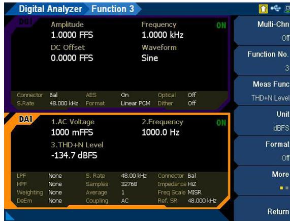
**Figure 4-22** Digital Analyzer > Functions > THD+N Level menu page 1
