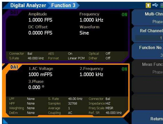
Figure 4-46 Digital Analyzer > Functions > Phase menu page
