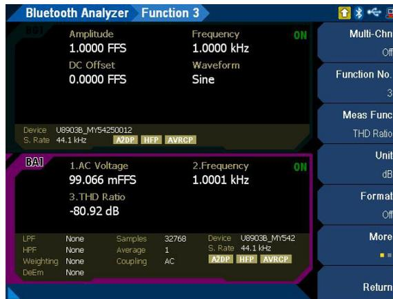
Figure 4-29 Bluetooth Analyzer > Functions > THD Ratio menu page 1
