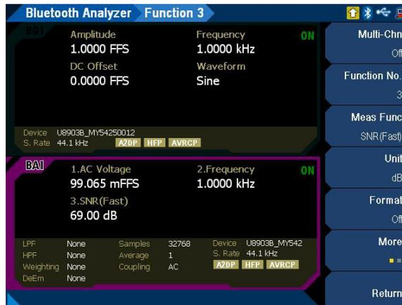
Figure 4-41 Bluetooth Analyzer > Functions > SNR (Fast) menu page 1
