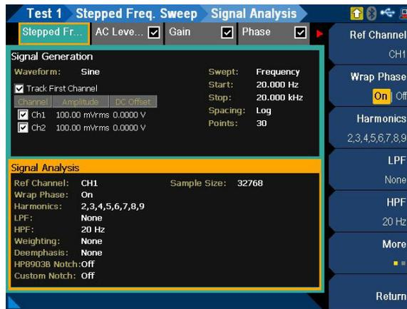
**Figure 7-38** Stepped Frequency Sweep > Signal Analysis settings menu page
