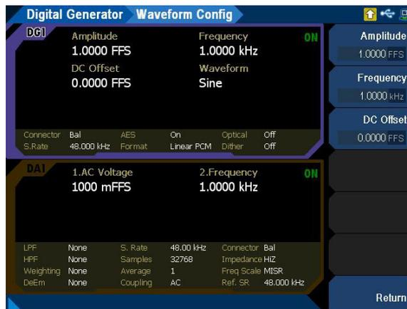
**Figure 3-5** Digital Generator > Waveform Config menu page (sine waveform)
