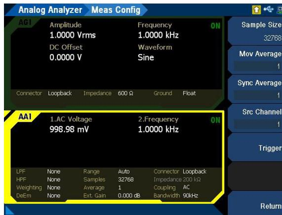
**Figure 4-56** Analog Analyzer > Meas Config menu page 1
