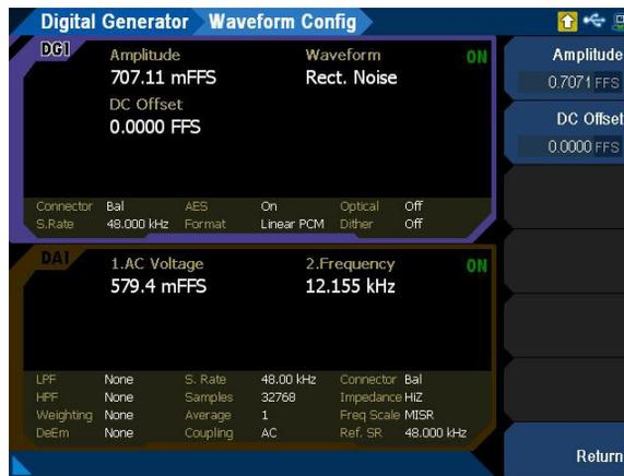
Figure 3-26 Digital Generator > Waveform Config menu page (Rectangular noise)
