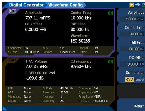
**Figure 3-20** Digital Generator > Waveform Config menu page (IEC 60268 waveform)
