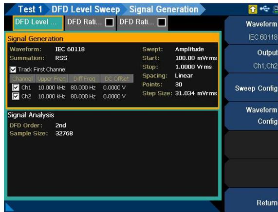
**Figure 7-49** DFD Level Sweep > Signal Generation settings menu page
