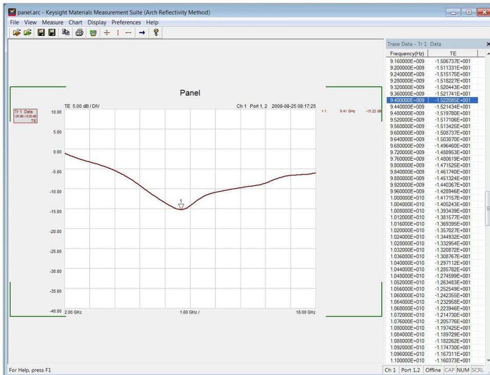
Figure 8. Example of arch reflectivity measurement results.
