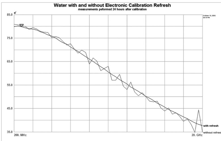
Figure 14. Water with and without electronic calibration refresh
