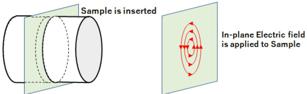
**Schematic diagram of a split cylinder resonator.** The split cylinder resonator is simply two metal cylinders (grey) cut in the middle to allow for a sample (green).
