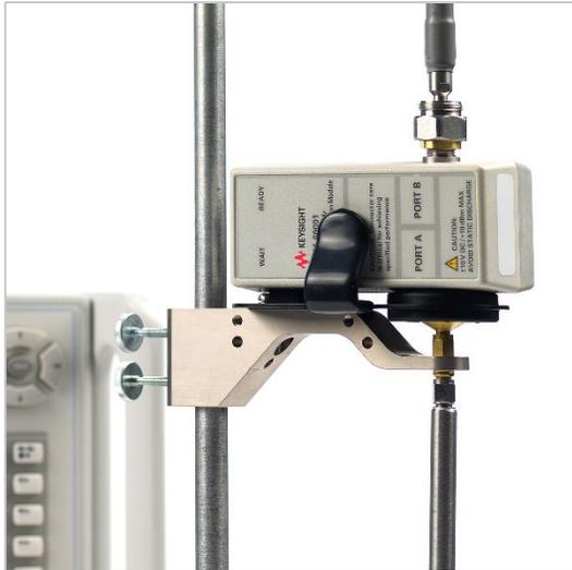
Figure 13. Ecal module connected in line for electronic
