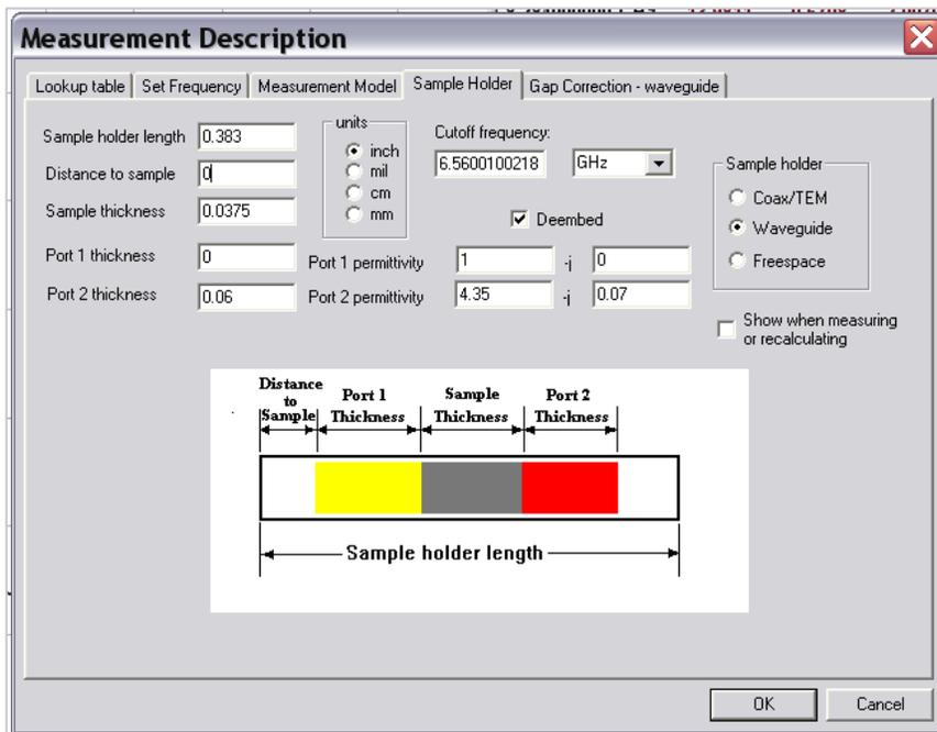
Figure 6. Sample holder definition screen with de-embedding
