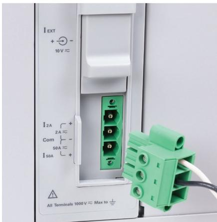
Figure 17. Direct current input connector
