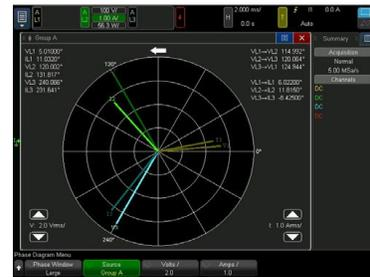
Figure 4. Phasor diagram for phase relationship analysis
