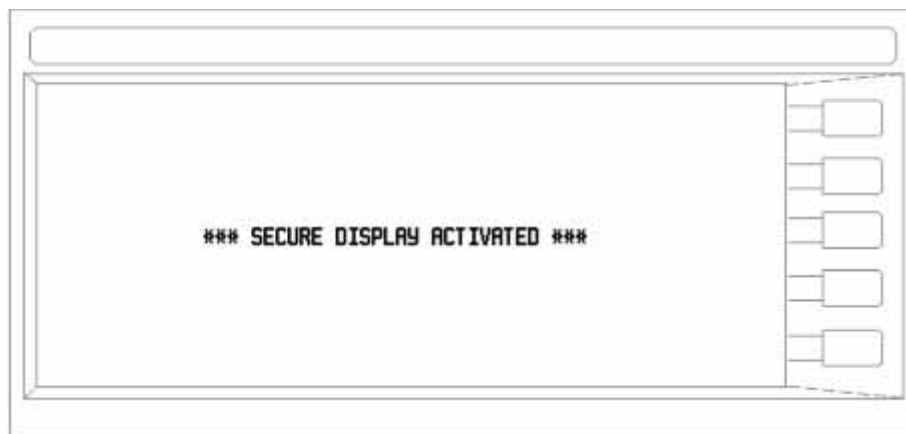
Figure 6-1 Signal Generator Screen with Secure Display Activated
