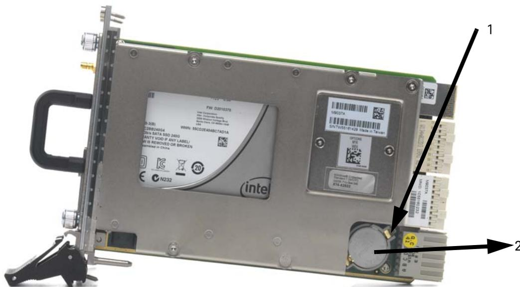
**Figure 14** Replacing the Battery
