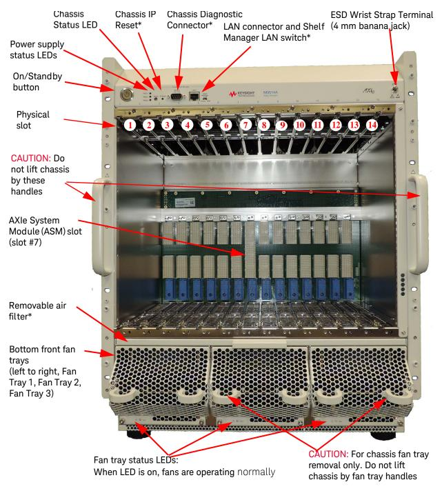
\* For detailed information, refer to the *M9514A and M9521A User Guide*. The DB-9 connector on the top front panel of the chassis labeled "Service Use Only" is for internal Keysight use only. There is no user diagnostic, troubleshooting, or service information available from this connector. Default Shelf Manager LAN switch position is to the right, ASM.
