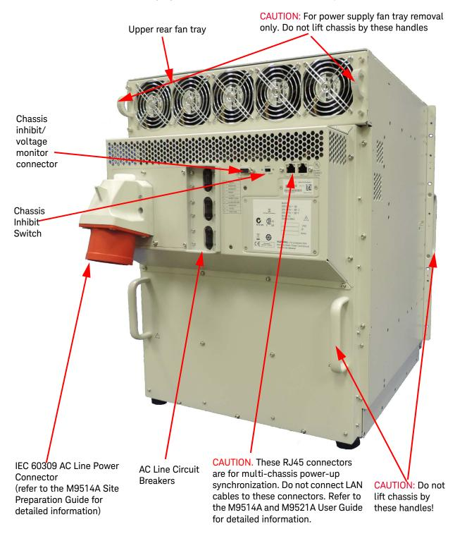
The following figure shows the M9514A chassis rear panel.
