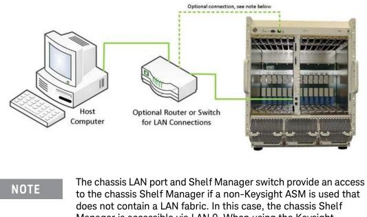
does not contain a LAN fabric. In this case, the chassis Shelf Manager is accessible via LAN 0. When using the Keysight M9521A ASM, the LANO connector is not used and the Shelf Manager LAN switch should remain in the default ASM (right) position.
