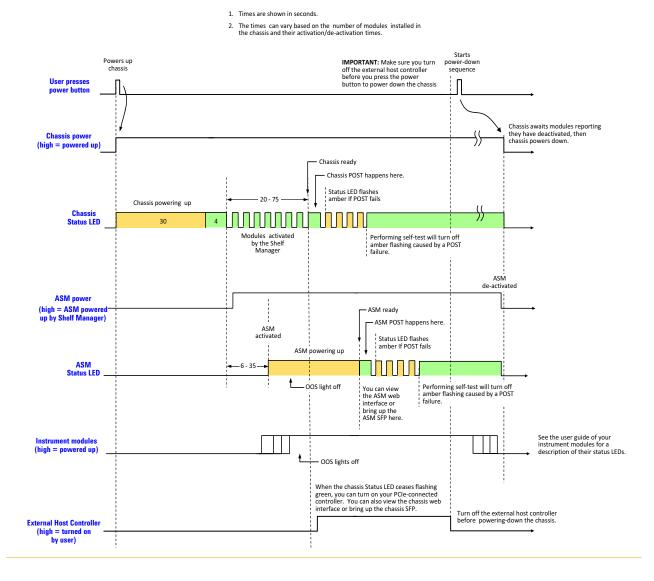
In brief, the external host pc must be off whenever the chassis is powered up or down. Because modules are not hot-swappable, the chassis must be powered down before modules are added or removed.
