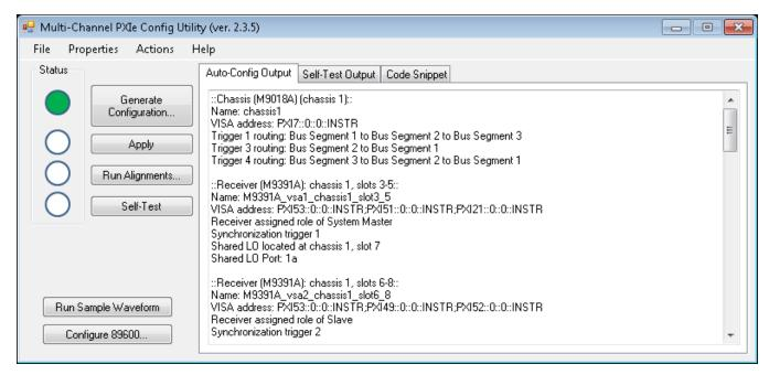
After clicking the 'Apply' button, the Config Utility will route the backplane trigger lines to the M9018A chassis and configure the [M9300A reference modules based on your configuration.
