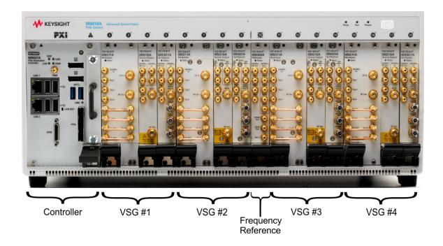
The recommended multiple PXI VSG system is configured as follows:
