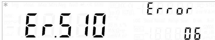
Press [▼] again to read the remaining errors. The error queue is automatically cleared when all errors have been read (primary display shows “nonE”).
