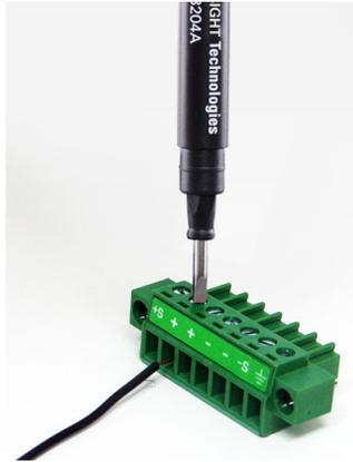
*Do not use the shield as one of the sensing conductors.* Ground the shield at the U3606B end only. The other end of the shield should be left unconnected. Observe the polarity when connecting the sensing leads to the load. You can connect the output leads to either one of the two + or - terminals. They are internally shorted.
