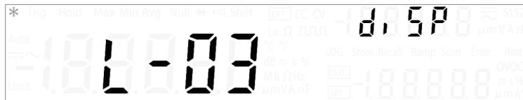
Press [ $\Delta$ ] or [ $\nabla$ ] to cycle between the available brightness levels (L-01, L-02, or L-03).
