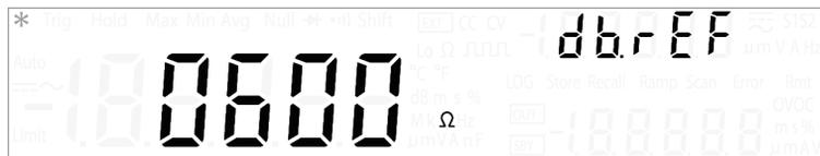
The dBm function is logarithmic, and is based on a calculation of power delivered to a reference resistance, relative to 1 mW. The following procedure shows you how to select an appropriate dBm reference resistance value. The factory default dBm reference resistance value is 600  $\Omega$ .
