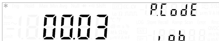
Press [ $\Delta$ ] or [ $\nabla$ ] to cycle between the interface board (Iob), source board (Sb), and measurement board (Mb) program code revisions.
