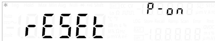
The following procedure shows you how to enable or disable the automatic recall of the power-off state when the power is turned on. For remote interface operation, refer to the `MEMORY: STATE: RECALL: AUTO` command in the *U3606B Programmer's Reference*.
