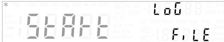
If “StArt” is selected, the U3606B will exit the Utility menu immediately and begin the data logging operation. The LOG annunciator turns on for the entire duration of the data logging operation.
