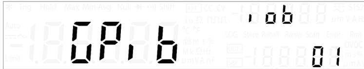
Press [ $\Delta$ ] or [ $\nabla$ ] to change the remote interface connection (GPIB, U-CdC, or U-tMC).
