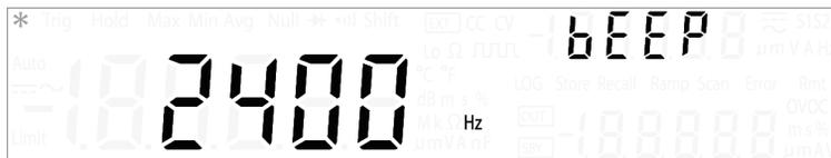
Normally, the U3606B beeps whenever certain conditions are met (for example, the U3606B beeps when a stable reading is captured in reading hold mode). The beep driving frequency is set to “3840 Hz” by default, but may be disabled through the front panel.
