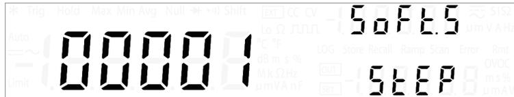
The U3606B allows you the option of soft starting the DC power supply output. You can select a value from 1 to 10000 steps for the soft start output. This feature is useful to start a DC motor. The factory default soft start step value is 1.
