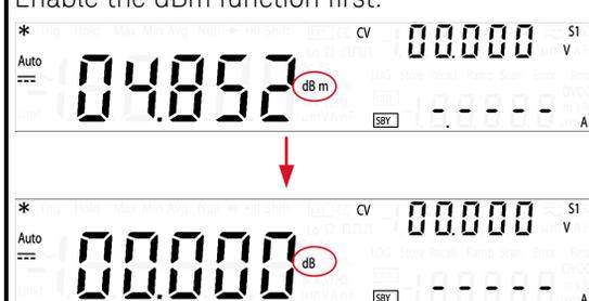
The first displayed reading is always precisely 00.000 dB.
