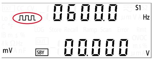
The digital display shows a square wave icon circled in red, indicating the selected function. The display shows 06000.0 and 00000.0.
