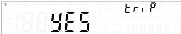
The OVP and OCP features depend on the output protection state function. The output protection state must be enabled for the OVP and OCP features to be active in the circuit. Disabling the output protection state will deactivate both the OVP and OCP features even if a trip level is set for either the OVP or OCP.
