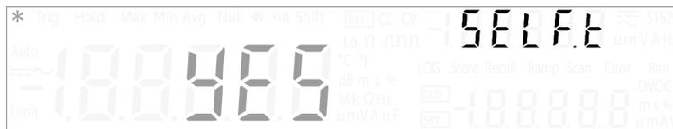
Press [ $\Delta$ ] or [ $\nabla$ ] to select “YES” and then press [**Shift**] > [**Save**] to save. The instrument will automatically exit the Utility menu and execute the self-test.
