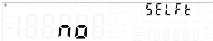
A power-on self-test occurs immediately when you turn on the instrument. This limited test assures you that the U3606B is operational.
