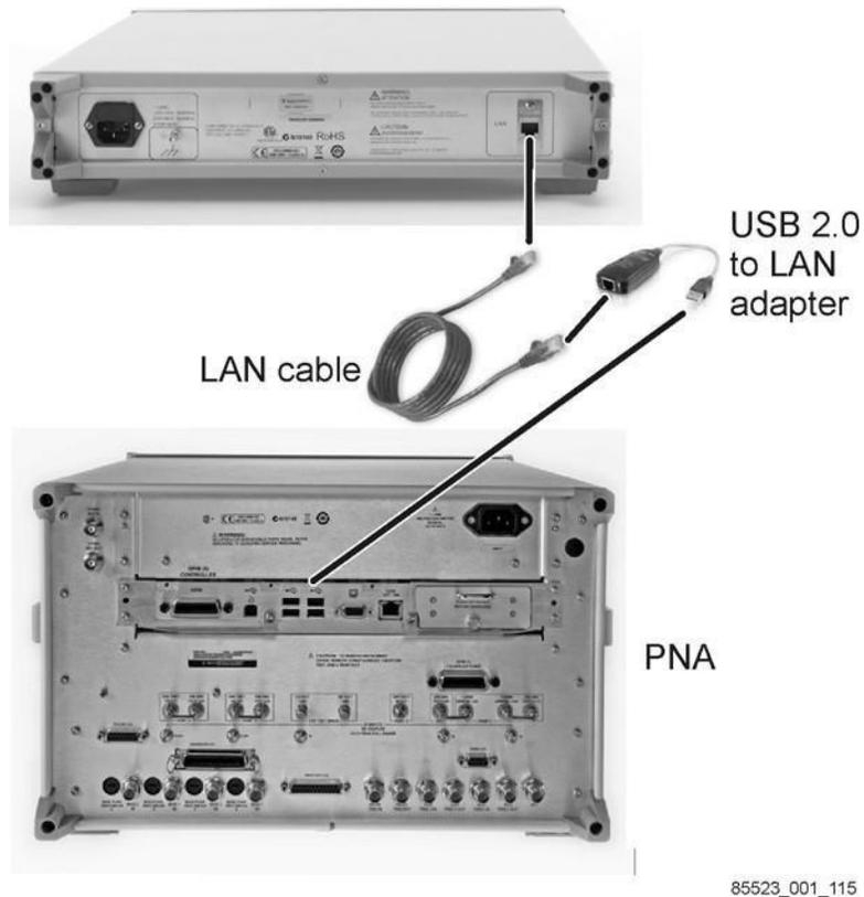
1. As shown in the graphic above, connect a LAN cable (not included) to the rear of the 85523B CalPod Controller and connect the other end to the USB 2.0 to LAN adapter (part number 0960-2955).
