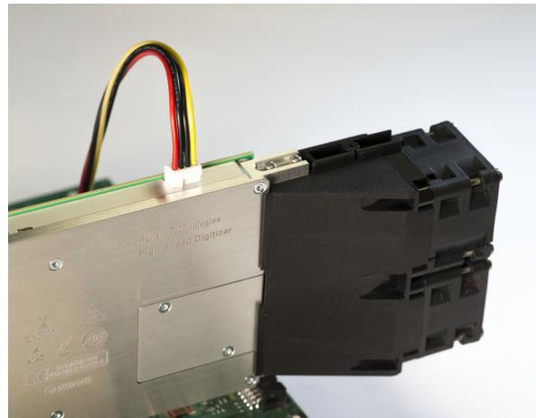
**CAUTION** Be careful there is no mechanical part of the PC that could damage the power adaptor cable.
