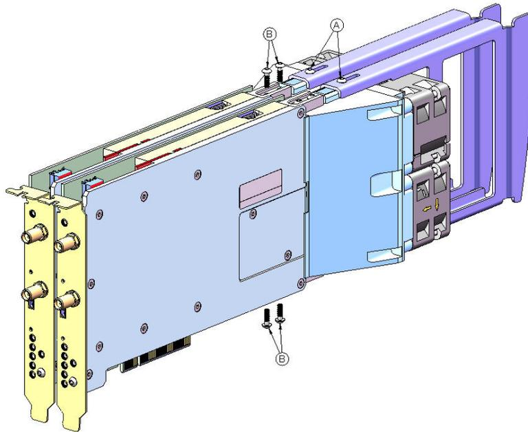
Diagram showing U5303A fan/support assembly fixings .
