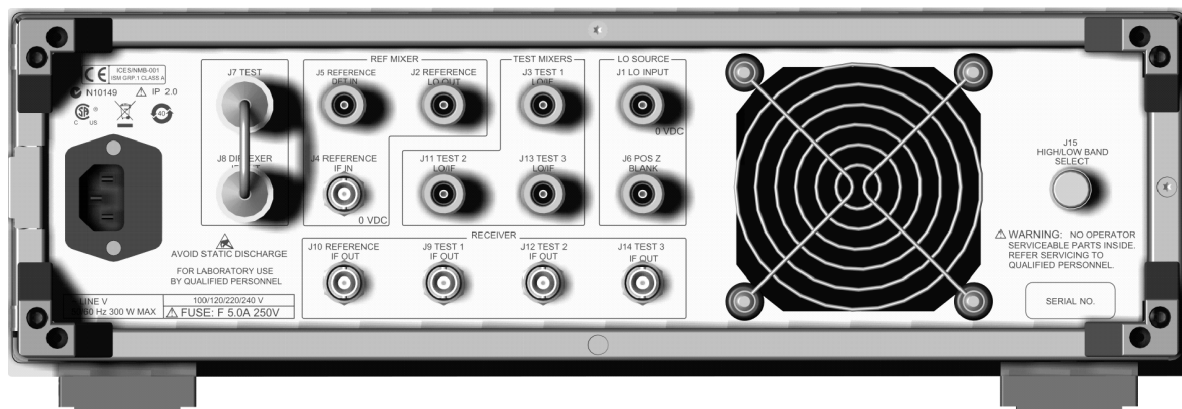
Figure 2-4 85309B Rear Panel Features (Option 402 and 002 without J15)
