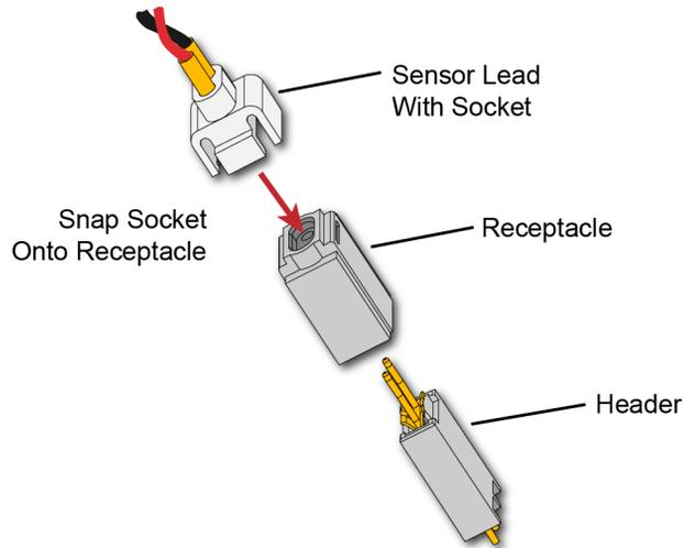
Figure 17 Socketed Lead Snaps Onto the MBB Receptacle
