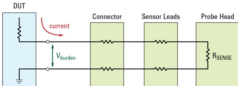
Figure 20  $V_{\text{burden}}$  Developed Across Probing Components
