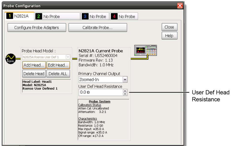
Figure 22 Infiniium Dialog Box With N2825A Heads
