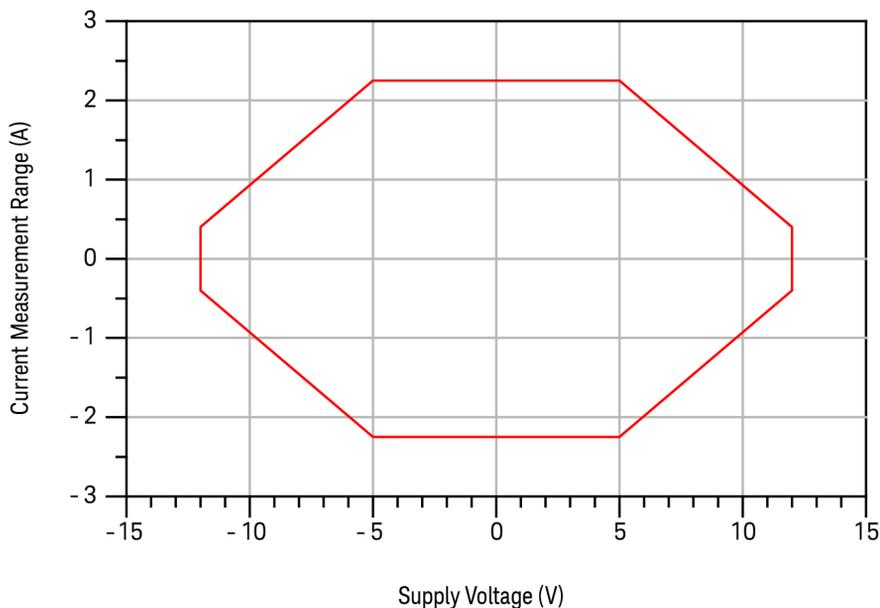
Figure 38 N2822A zoomed-in current measurement range versus supply voltage
