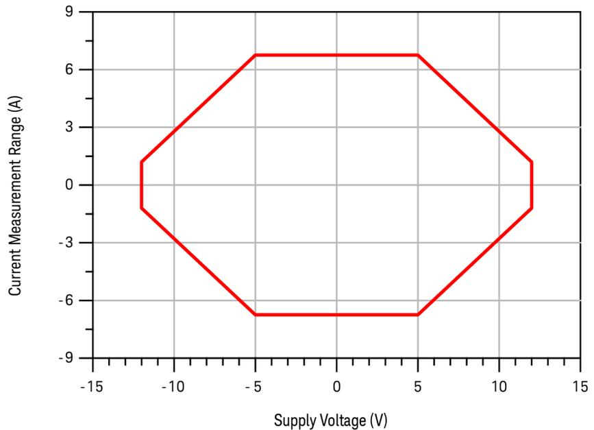
Figure 41 N2825A zoomed-out current measurement range versus supply voltage
