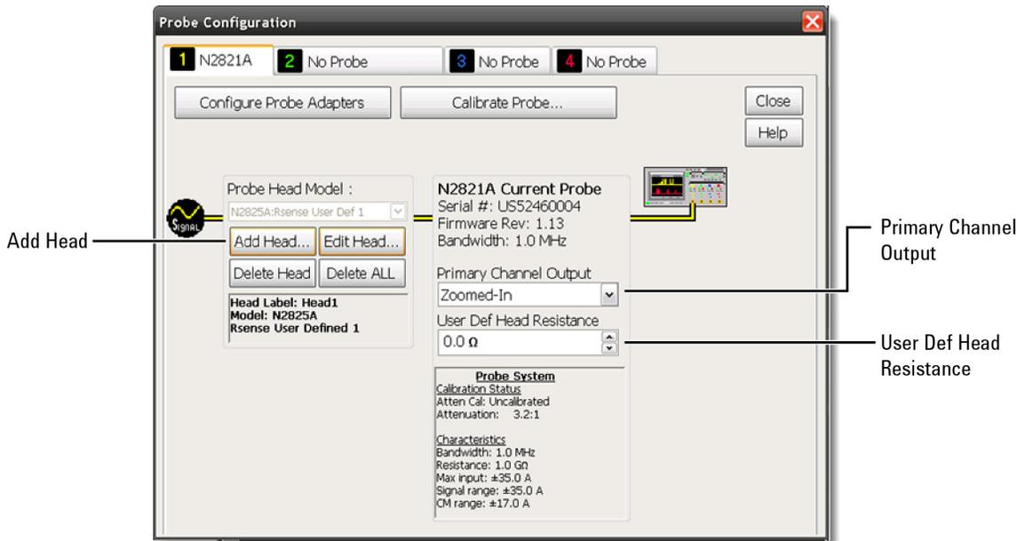
Figure 9 Probe Configuration Dialog Box (N2821A Probe)
