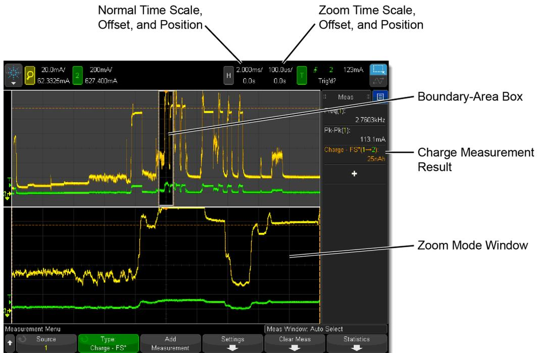
Figure 14 Full Screen Charge Measurement with Zoom Mode
