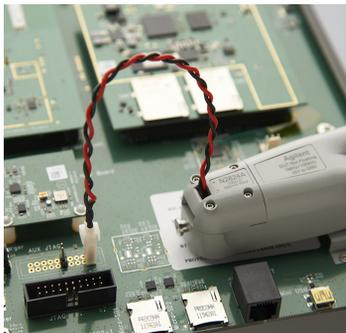
In this chapter, you'll learn how to connect the probe to the oscilloscope and how to perform several measurements. The probe accessories are very flexible and can be configured to match your unique probing requirements regarding convenience versus accuracy.
