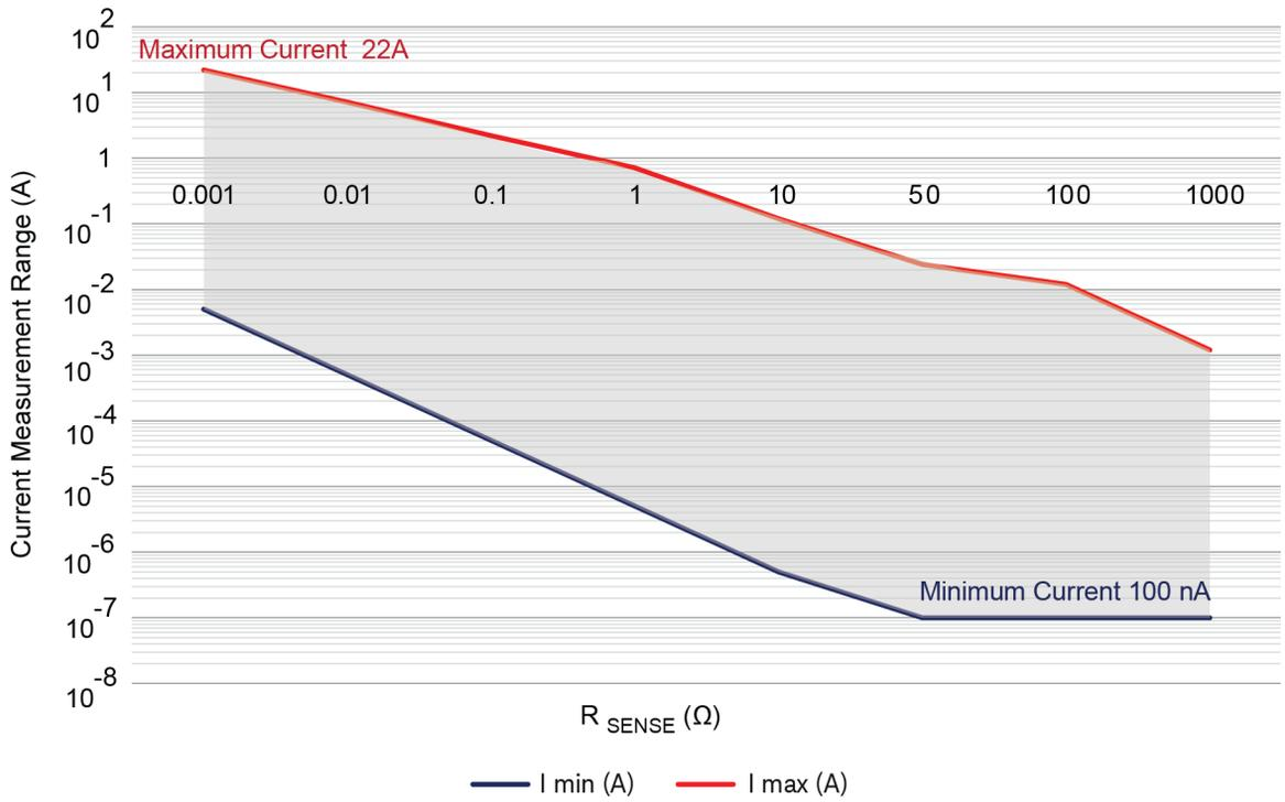
Figure 36 Minimum/maximum current measurement range with N2825A head, 500 mW  $R_{sense}$ , solder attached, high resolution mode on
