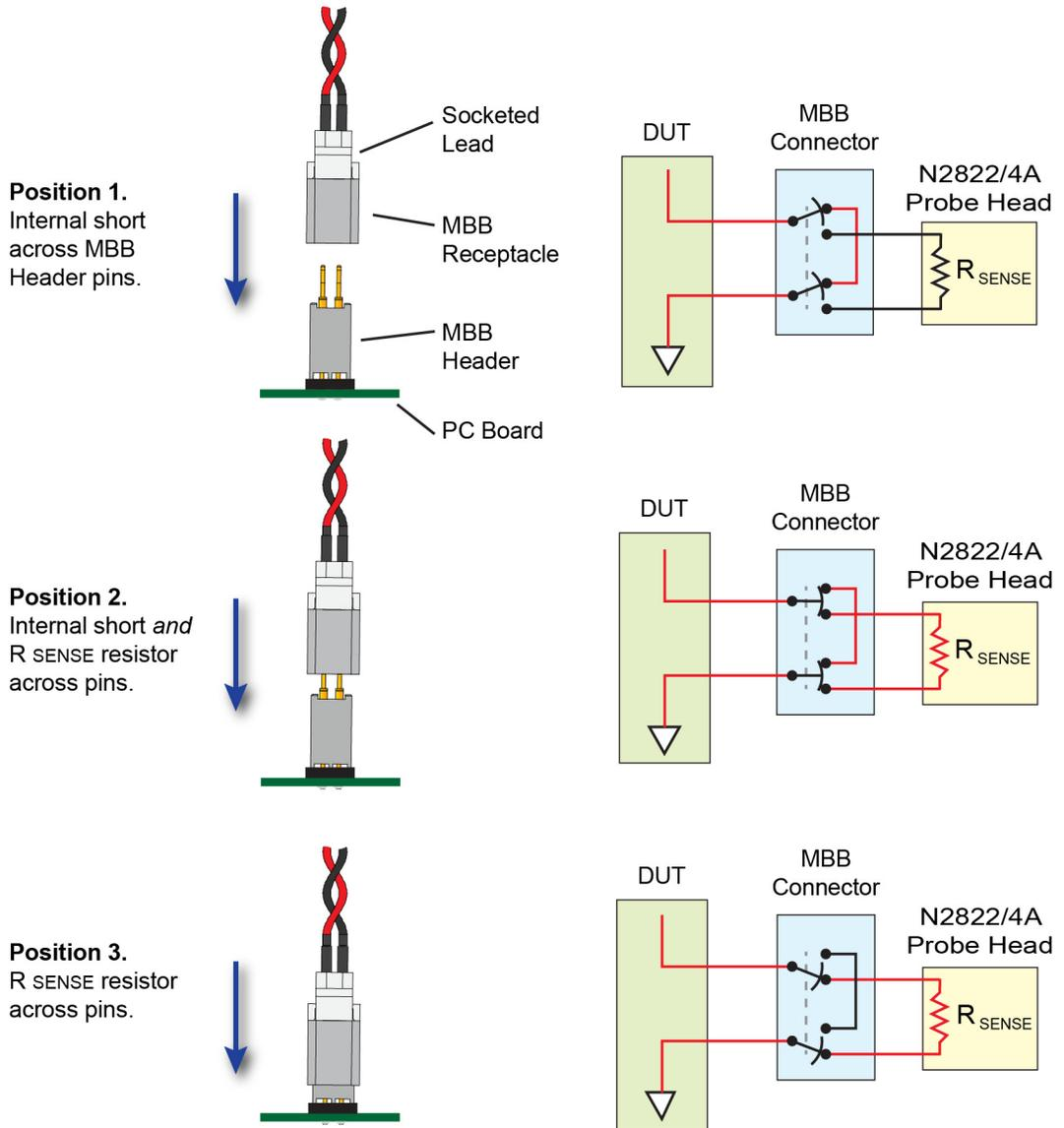
Figure 18 Connecting the MBB Connector with N2822/4A Head
