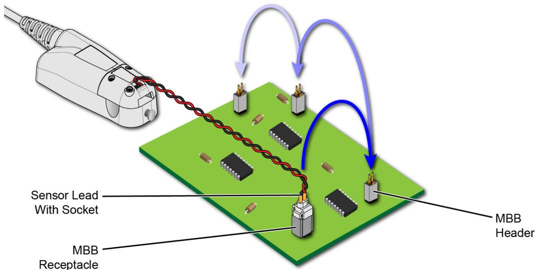
Figure 16 Probing with MBB Connector on DUT
