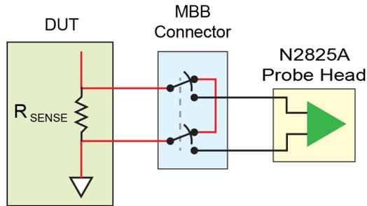
Figure 19 MBB Connector With N2825A User-Defined Head
