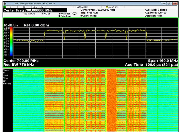
Figure 9. Spectral analysis of an LTE signal where, without demodulation, you can see the signal, control and synch structures are present.
