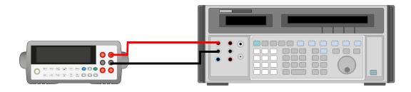
4-W resistance with compensation (For range 100  $\Omega$  ~ 100 k $\Omega$ )
