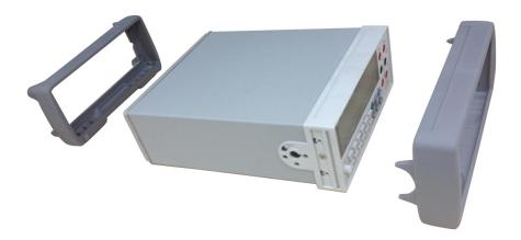
Remove the rear bezel. Loosen the two captive screws in the rear bezel and remove the rear bezel.
