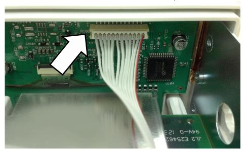
**8** Disconnect the individual front panel wires as shown in the figure below:
