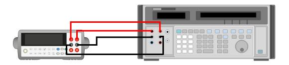
4-W resistance without compensation (For range 1 M $\Omega$  ~ 100 M $\Omega$ )
