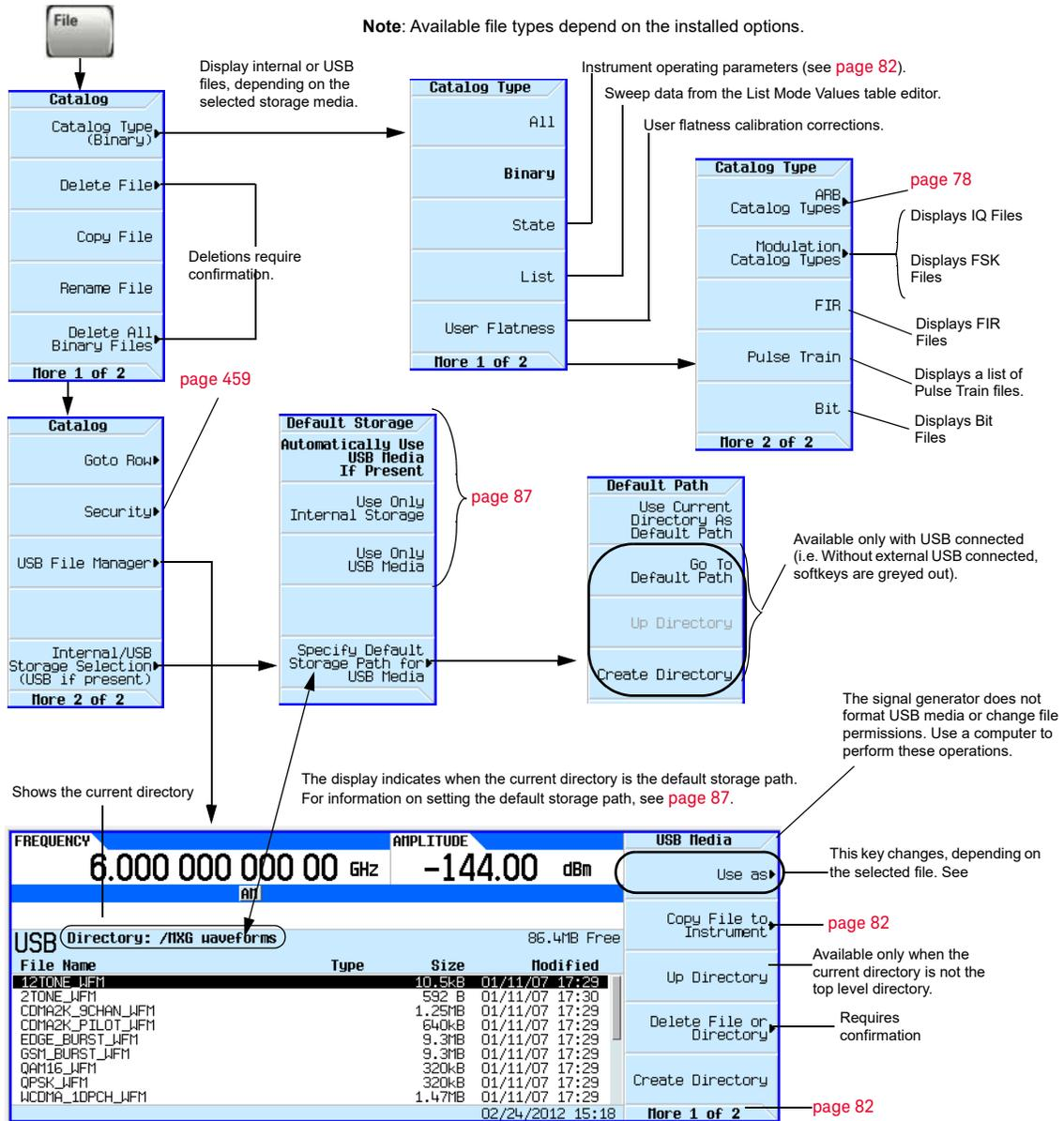
When you connect USB media to the instrument, the signal generator displays the USB Media menu and the message **External USB Storage attached**. When you disconnect the USB media, the message **External USB Storage detached** displays. When you open the External Media menu without USB media connected, the signal generator displays the message **External Media Not Detected**.
