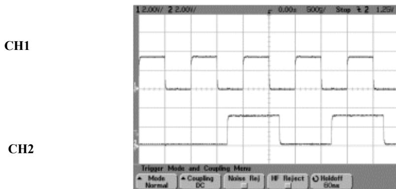
CH1: BER TEST OUT (pin 17 of AUX I/O connector)
