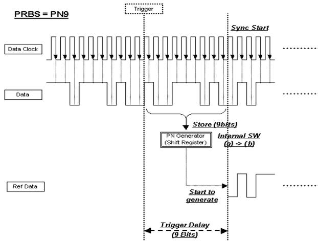
In this example, the triggering sequence is where the trigger delay is active with a cycle count.
