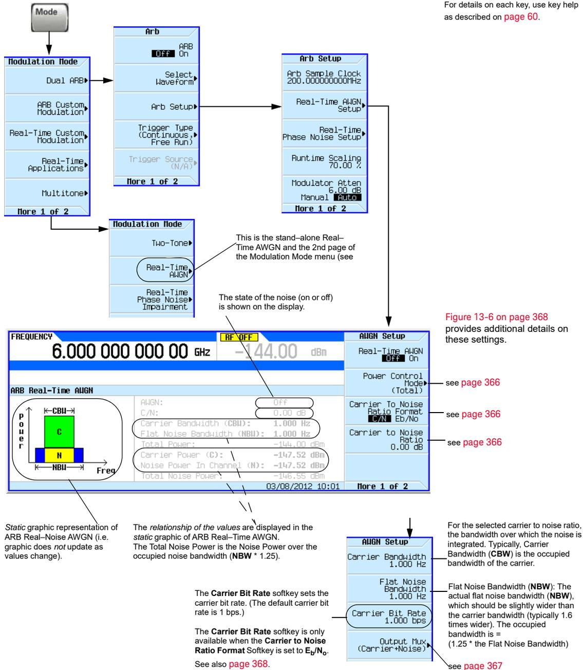
Figure 13-2 Real Time I/Q Baseband AWGN - Power Control Mode Softkeys
