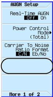
Whether a softkey is available depends on the **Carrier to Noise Ratio Format** softkey setting (e.g. C/N or  $E_b/N_0$ ).
