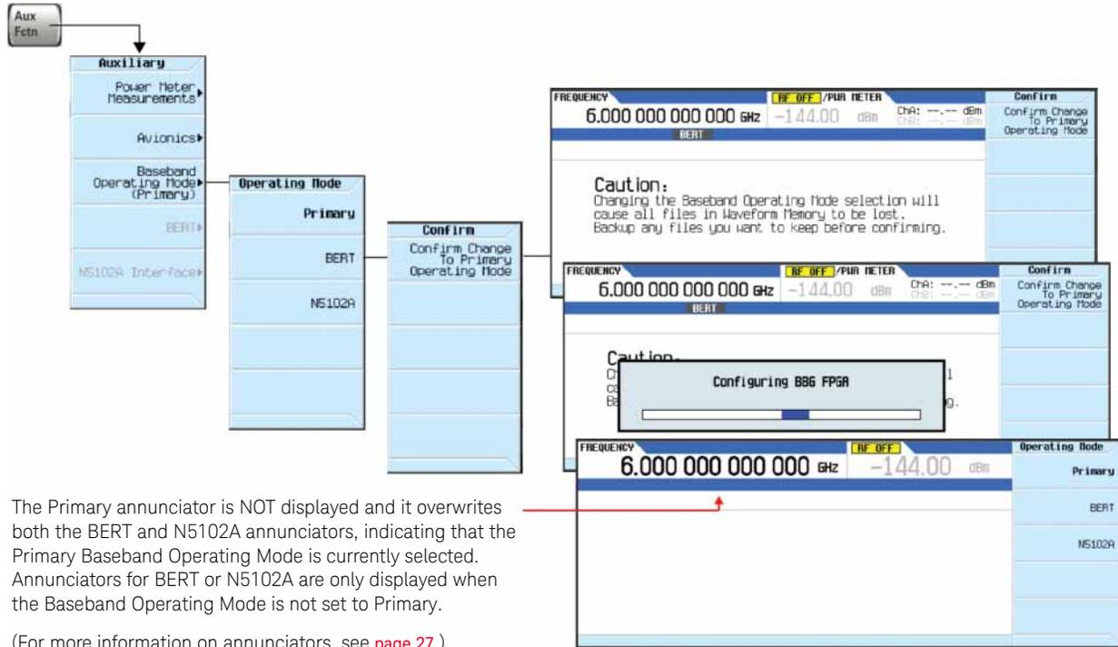
The Primary annunciator is NOT displayed and it overwrites both the BERT and N5102A annunciators, indicating that the Primary Baseband Operating Mode is currently selected. Annunciators for BERT or N5102A are only displayed when the Baseband Operating Mode is not set to Primary.
