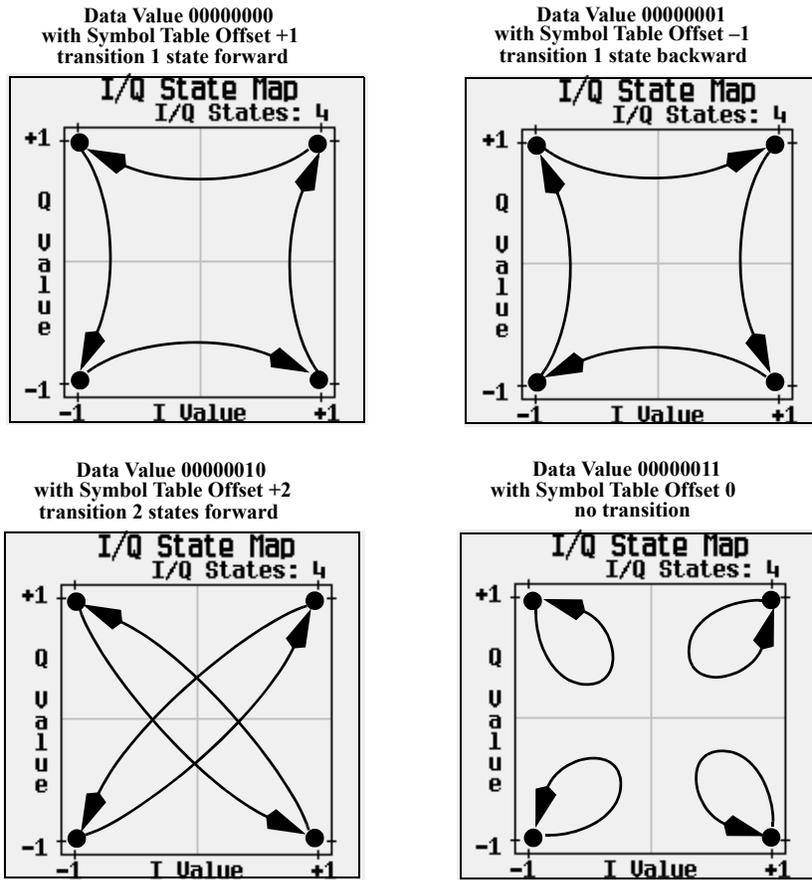
When applied to the user-defined default 4QAM I/Q map, starting from the 1st symbol (data 00), the differential encoding transitions for the data stream (in 2-bit symbols) 0011100001 appear in the following illustration.
