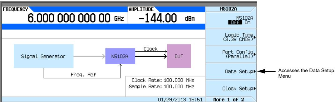
This softkey menu accesses the various parameters that govern the data received by the signal generator. The status area of the display shows the number of data lines used for both I and Q along with the clock position relative to the data. **Figure 10-22** shows the data setup menu structure.
