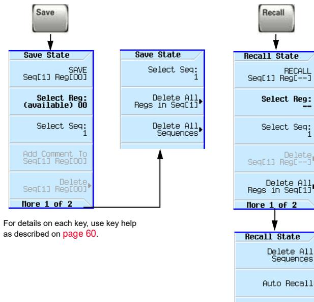
When saved to the signal generator, instrument settings (states) save to instrument state memory\*. Instrument state memory is divided into 10 sequences (0 through 9); each sequence comprises 100 registers (00 through 99).
