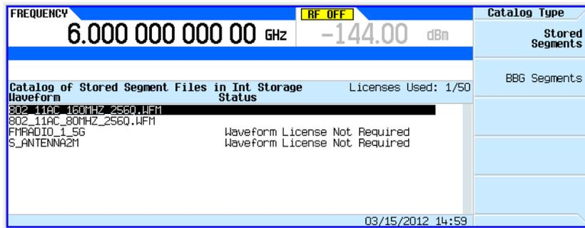
This softkey displays a catalog of the waveform segments stored in the **Int Storage** or **USB Media**.
