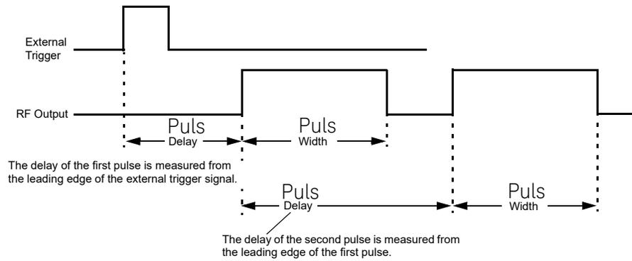
Figure 7-3 Trigger Doublet
