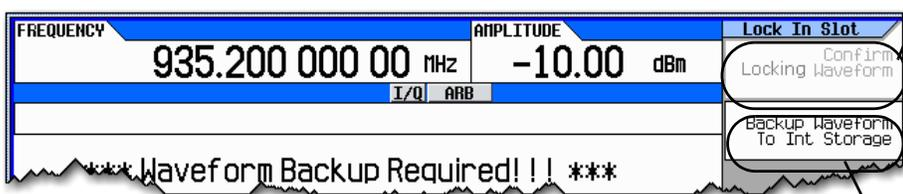
Press this softkey to store the waveform into the internal storage and to activate the **Confirm Locking Waveform** softkey.
