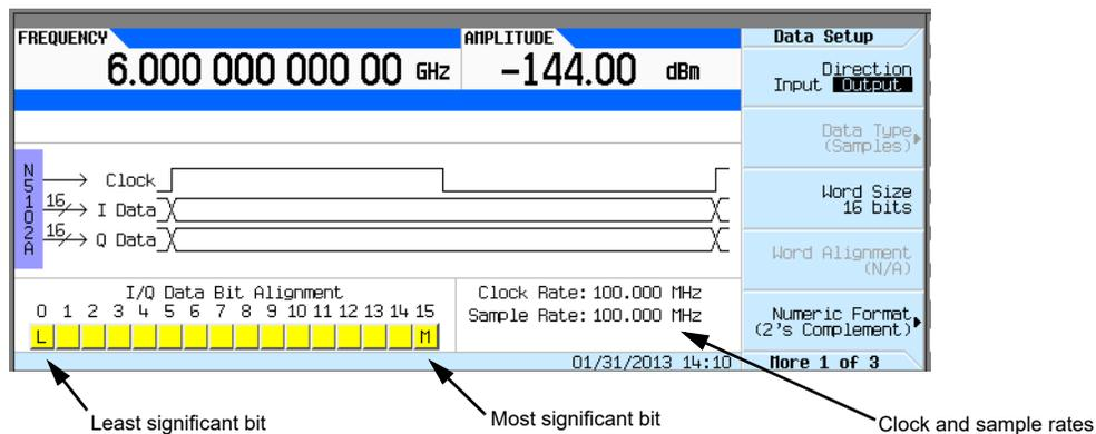
The N5102A module clock rate is set using the **Clock Rate** softkey and has a range of 1 kHz to 400 MHz. The sample rate is automatically calculated and has a range of 1 kHz to 200 MHz. These ranges can be smaller depending on logic type, data parameters, and clock configuration.
