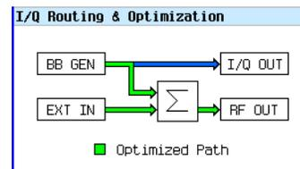
Notice that only the internal BBG (**BB GEN**) routes I and Q signals to the rear panel I and Q outputs.
