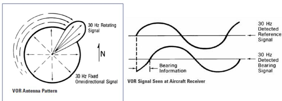
When using an X-Series signal generator with Option N5180302B Avionics License to simulate VOR signals, the 30 Hz reference signal (REF Freq) is placed on a sub-carrier of 9960 Hz (SubCarrier Freq) using frequency modulation with a peak deviation set to 480 Hz (REF Deviation). This frequency modulated sub-carrier is then amplitude modulated onto one of the VOR carriers (108.00 to 117.95 MHz). This makes the reference signal essentially an FM/AM multiplex signal.
