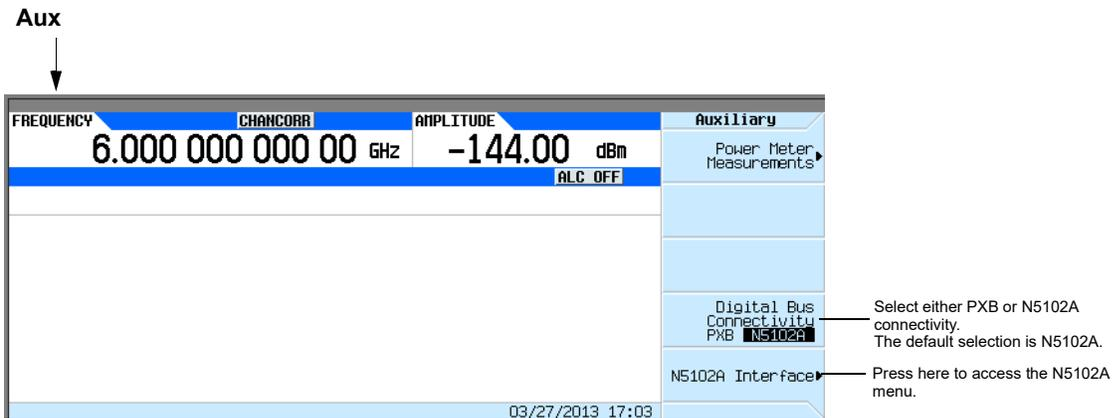
All parameters for the N5102A module are set with softkeys on the signal generator.
