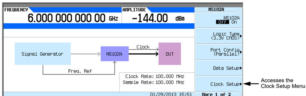
From this softkey menu, set all of the clock parameters that synchronize the clocks between the N5102A module and the signal generator. You can also change the clock signal phase so the clock occurs during the valid portion of the data. Figure 10-15 shows the clock setup menu.
