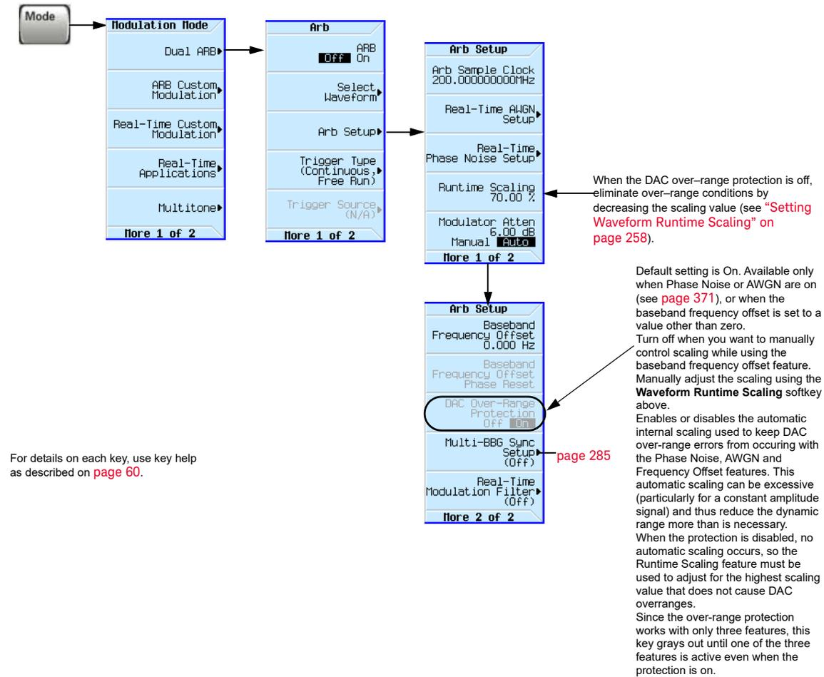
In the Dual ARB Player, to avoid excessive scaling or to just perform scaling manually, turn the feature off and use the **Waveform Runtime Scaling** softkey to eliminate DAC over-range conditions.
