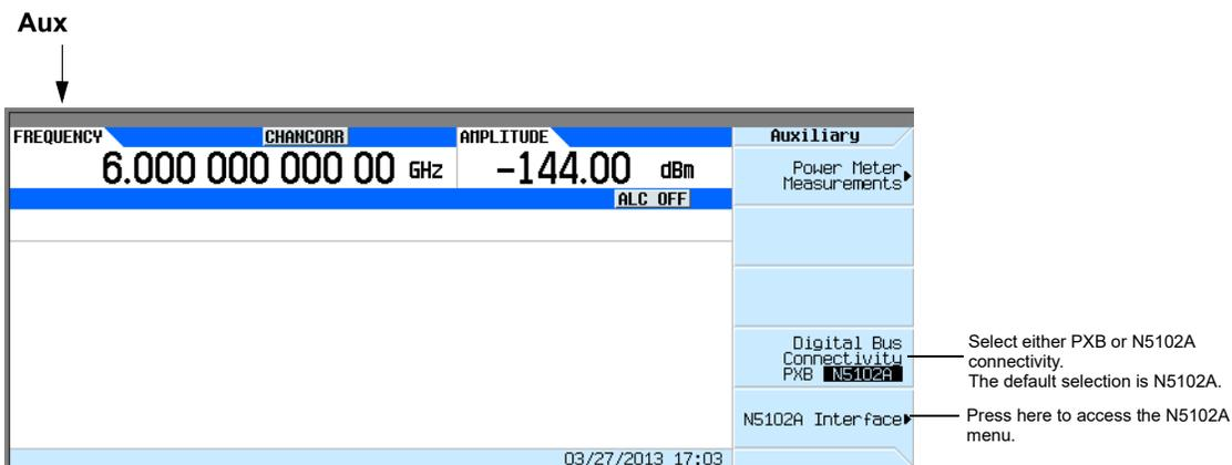
Press N5102A Interface to access the UI (first-level softkey menu shown in **Figure 10-10**) that is used to configure the digital signal interface module. Notice the graphic in the signal generator display, showing a setup where the N5102A module is generating its own internal clock signal. This graphic changes to reflect the current clock source selection.
