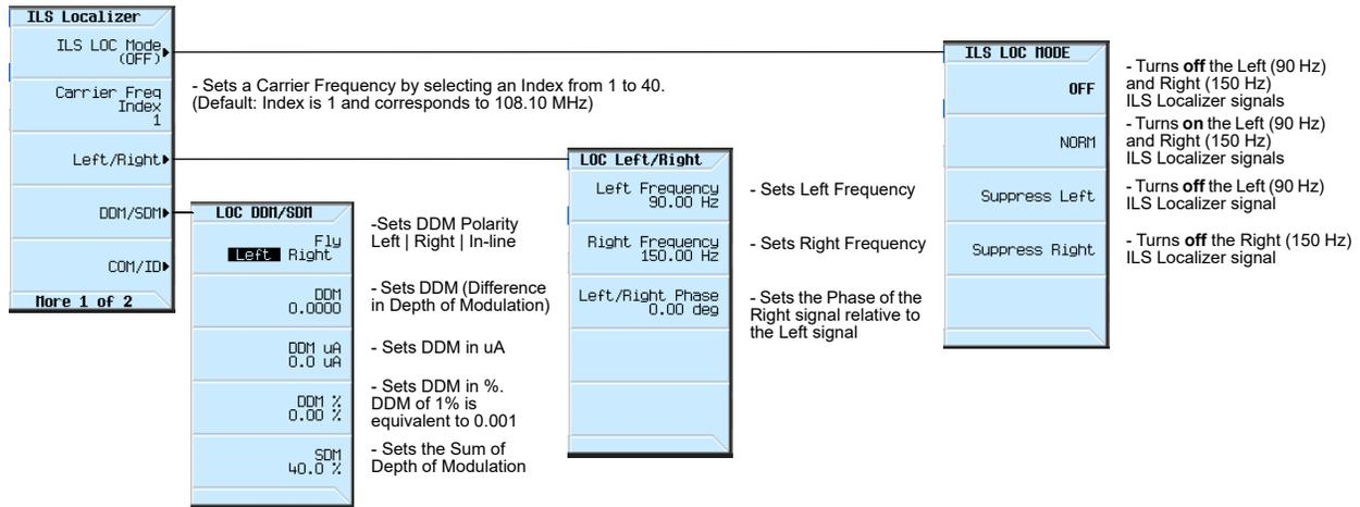
When testing an ILS [Instrument Landing System], the following ILS Localizer parameters can be set:
