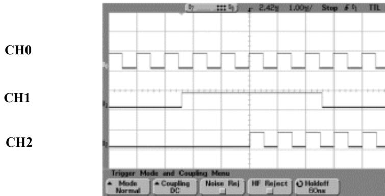
CH0: BER CLK IN (rear panel BNC connector labeled BB TRIG 1)
