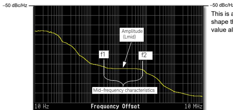
This is a plot of the unmodified phase noise shape that shows the location that each value alters.
