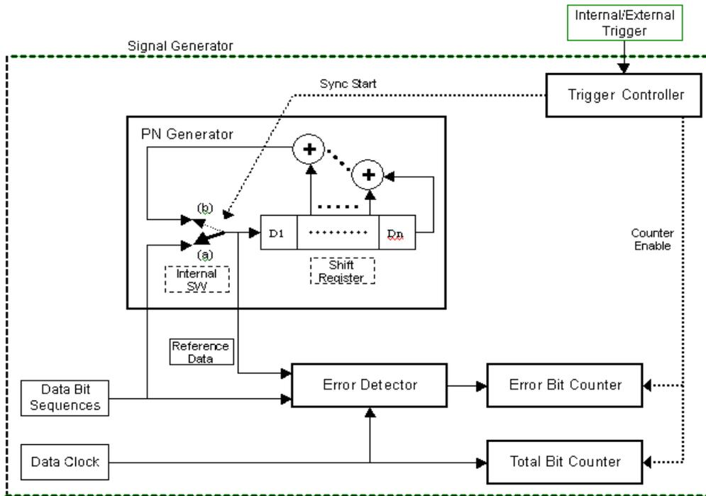
In this example, the triggering sequence is where you have an incoming data clock and data bit sequences, the trigger is active, and the BERT measurement begins. Refer to **Figure 12-8**.
