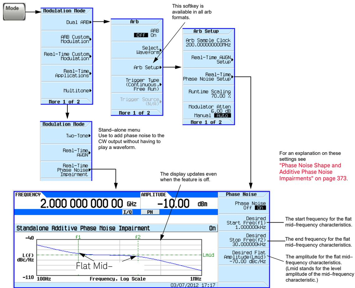
**NOTE:** The phase noise impairment is added to the base phase noise of the signal generator.
