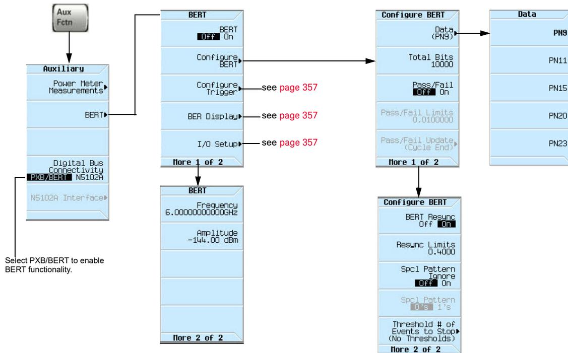
Figure 12-15 BERT I/O Setup Softkeys
