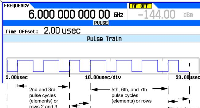
This is the initial pulse cycle (row 1) note that the On Time portion of this pulse is not showing due to the 2 us offset.
