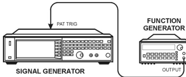
1. Connect the signal generator to the function generator as shown above.
