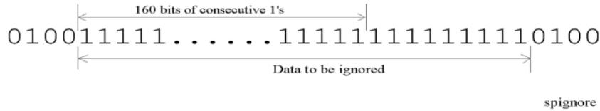
The 160 or more ignored bits can be anywhere in the PN sequence. The signal generator ignores these bits as error, but they are counted in the PN sequence bit count.
