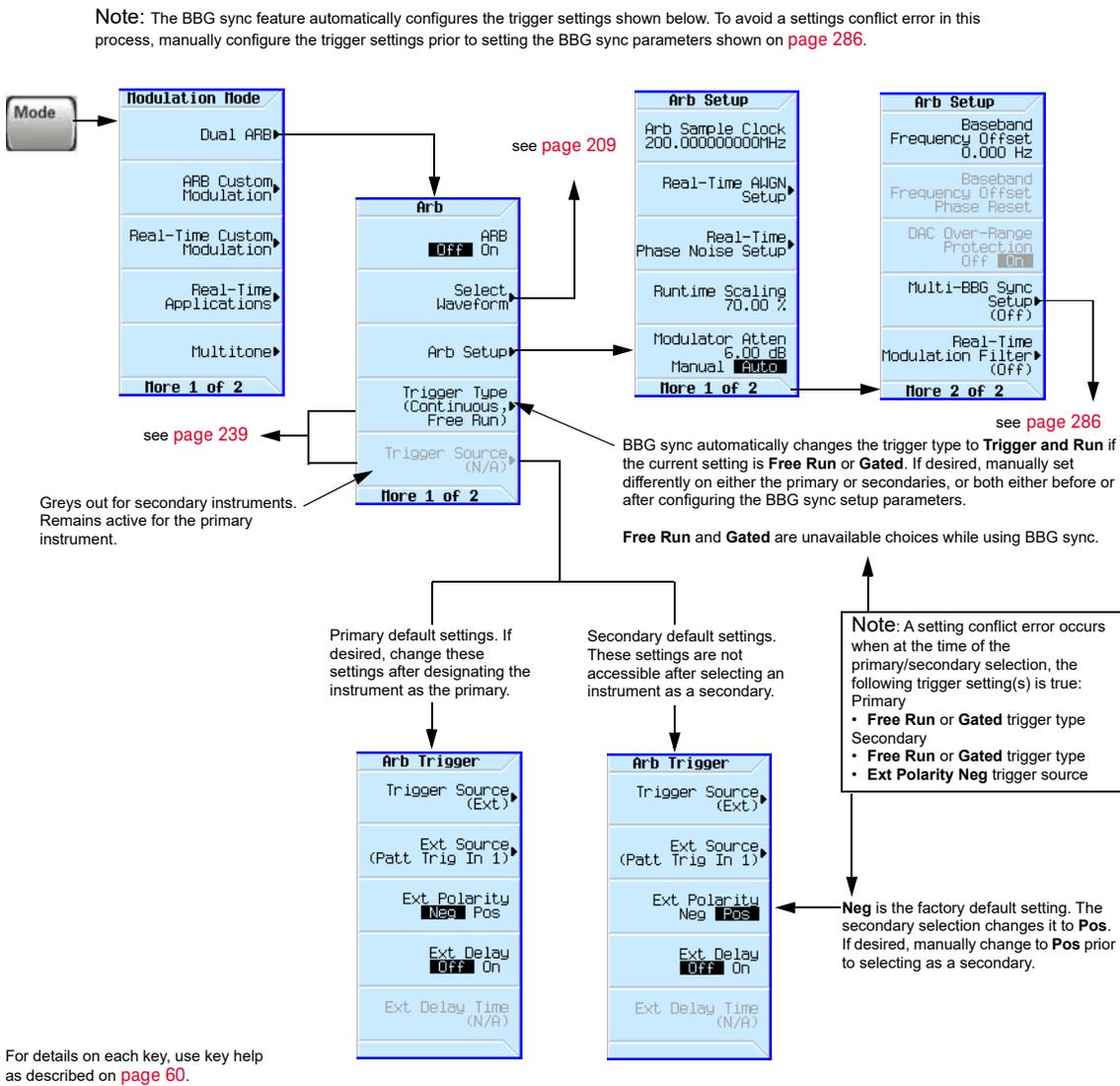
Figure 9-28 Multiple BBG Synchronization Front Panel Displays
