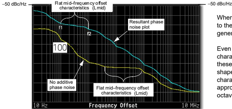
When turned on, this phase noise is added to the base phase noise of the signal generator.
