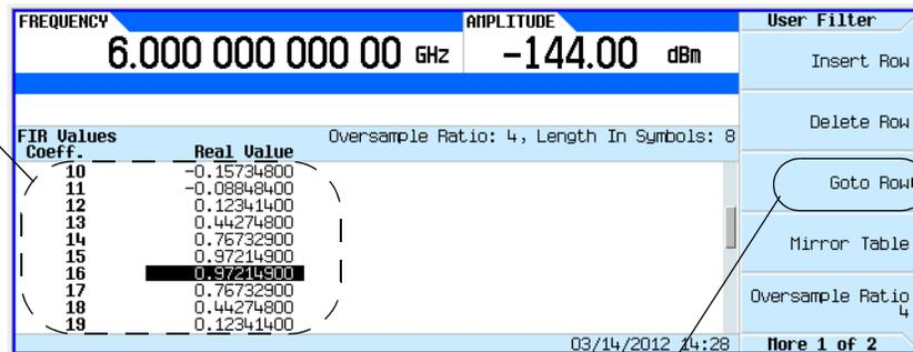
Use the Goto Row menu to move around and make changes to the FIR Values coefficient table.
