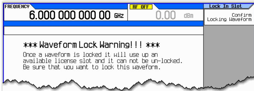
b. Press **Confirm Locking Waveform**.
