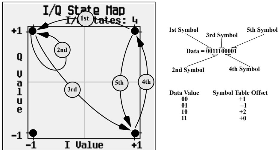
As you can see from the previous illustration, the 1st and 4th symbols, having the same data value (00), produce the same state transition (forward 1 state). In differential encoding, symbol values do not define location; they define the direction and distance of a **transition** through the I/Q State Map.
