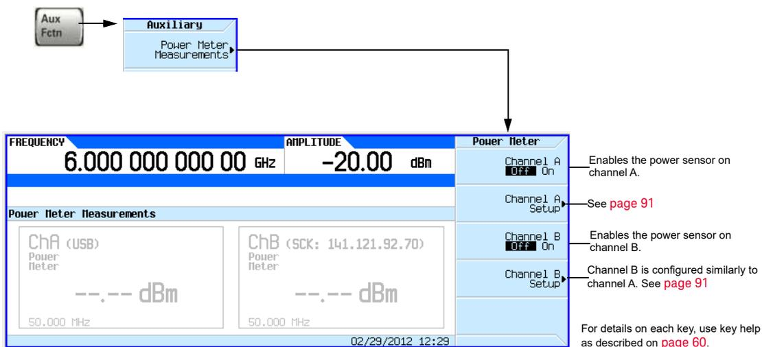
Figure 4-3 Configuring the Power Sensor Channels
