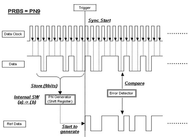
In this example, synchronization occurs after receiving a trigger.
