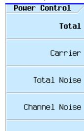
Selecting **Carrier** as the power control mode makes the carrier power and C/N independent variables while making the total power and total noise power dependent variables. The dependent variables total power and total noise power are set by the carrier power, C/N, and the rest of the Noise settings. The total power and total noise power change as any noise parameter is adjusted to keep the carrier power and the C/N at their last specified values.
