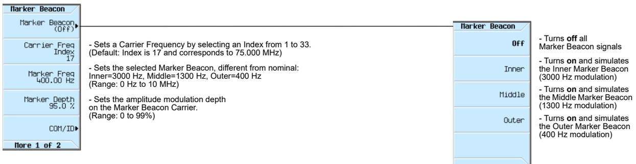
When testing an ILS [Instrument Landing System], the following ILS Marker Beacon parameters can be set:
