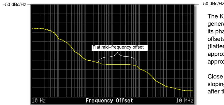
The Keysight X-Series vector signal generator demonstrates a definitive shape to its phase noise plot. The mid-frequency offsets are characterized by a leveling (flattening) of the phase noise amplitude from approximately a 3 kHz offset to approximately a 70 kHz offset.
