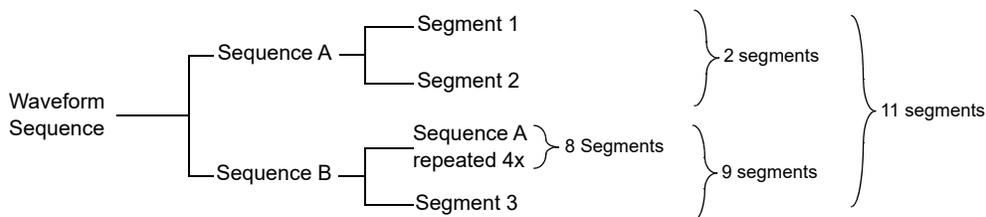
The maximum number of times that a nested sequence can repeat is based on the number of segments in the nested sequence and the remaining number of allowed segments (1,024). For example, with a sequence that contains 24 segments and one nested sequence with 4 segments, the nested sequence is limited to 250 repetitions:
