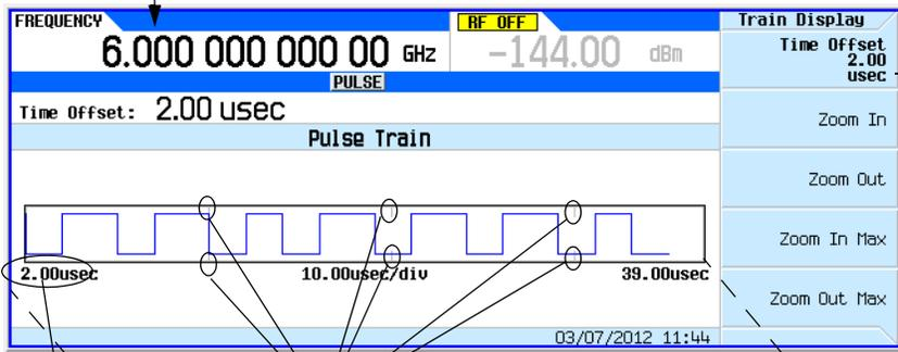
This softkey shifts the time offset from the left hand side of the display to the one specified. Increments and decrements are 1/20th of the visible pulse train.
