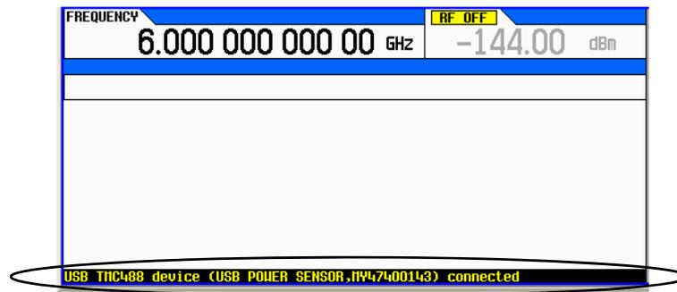
3. Press **Aux Fctn** > **Power Meter Measurements** > **Channel A Setup** > **Connection Settings** > **Connection Type** > **USB Device (None)** > **USB POWER SENSOR (MY47400143)**
