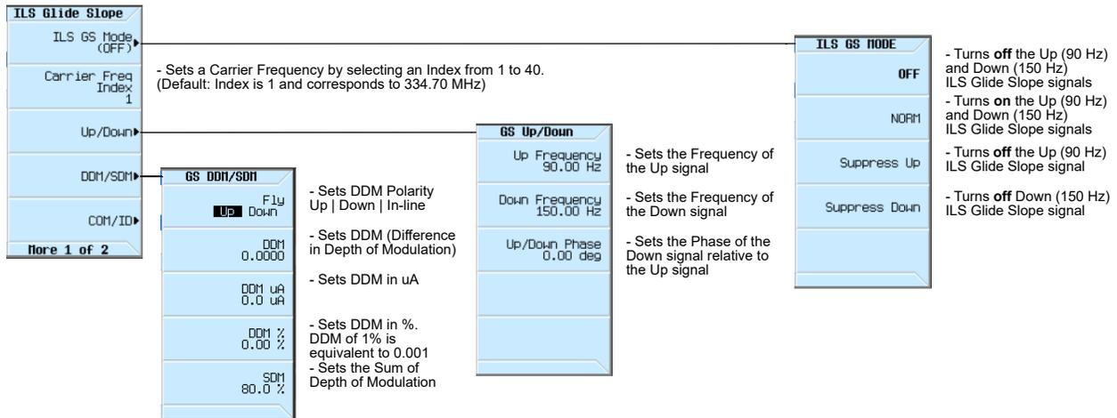
When testing an ILS [Instrument Landing System], the following ILS Glide Slope parameters can be set:
