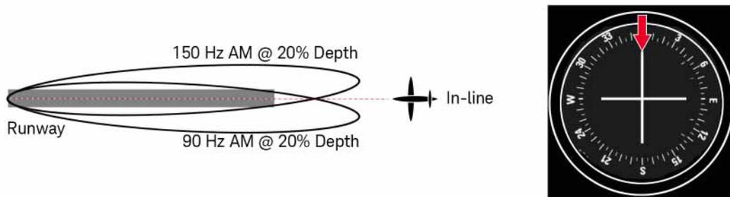
Figure 5-7 ILS Glide Slope: 334.70 MHz w/ 90 Hz AM (Up), 150 Hz AM (Down) @ 40%
