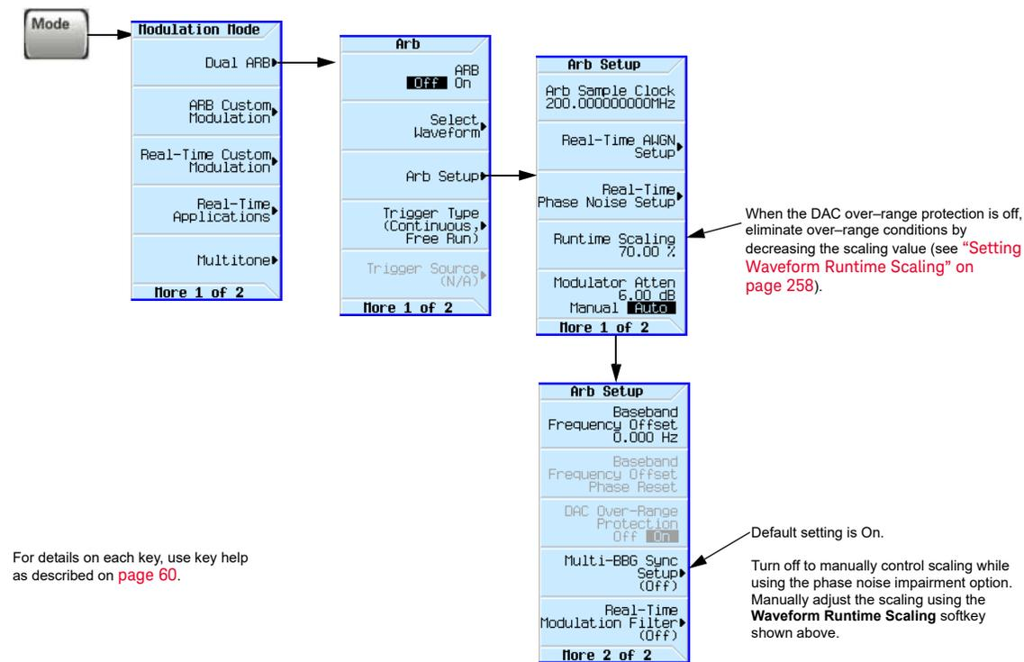
In the Dual ARB Player, to avoid excessive scaling or to just perform scaling manually, turn the over-range protection off and use the **Waveform Runtime Scaling** softkey to eliminate DAC over-range conditions.
