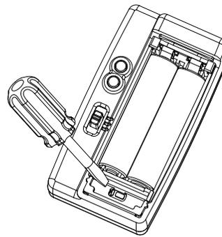
Use a flat-blade screwdriver to push the button-
