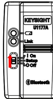
Set the slide switch to **Setup**.
