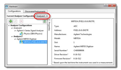
3. Review and configure the Measurement Setup Parameters as detailed in the document: M9703 Hardware Extension of 89600 VSA Software (M9703-90010).
