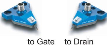
Prepare two RF probes to perform the RF measurement. The RF probe must have the signal line and the ground lines as shown in Figure 3-23. The signal line is to connect the gate or drain pad, and the ground lines are to connect the source/well pads. For the RF probe and its installation, consult your favorite prober vender. Figure 3-22 shows RF probes from Cascade Microtech, Inc.
