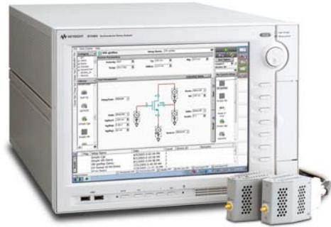
The B1500A also provides an intuitive graphical user interface, touch screen LCD panel, keyboard, and mouse for easy and effective measurement and analysis on the Windows environment. You can analyze a measurement result characteristics graph for example by using several tools such as markers, cursors, and lines.
