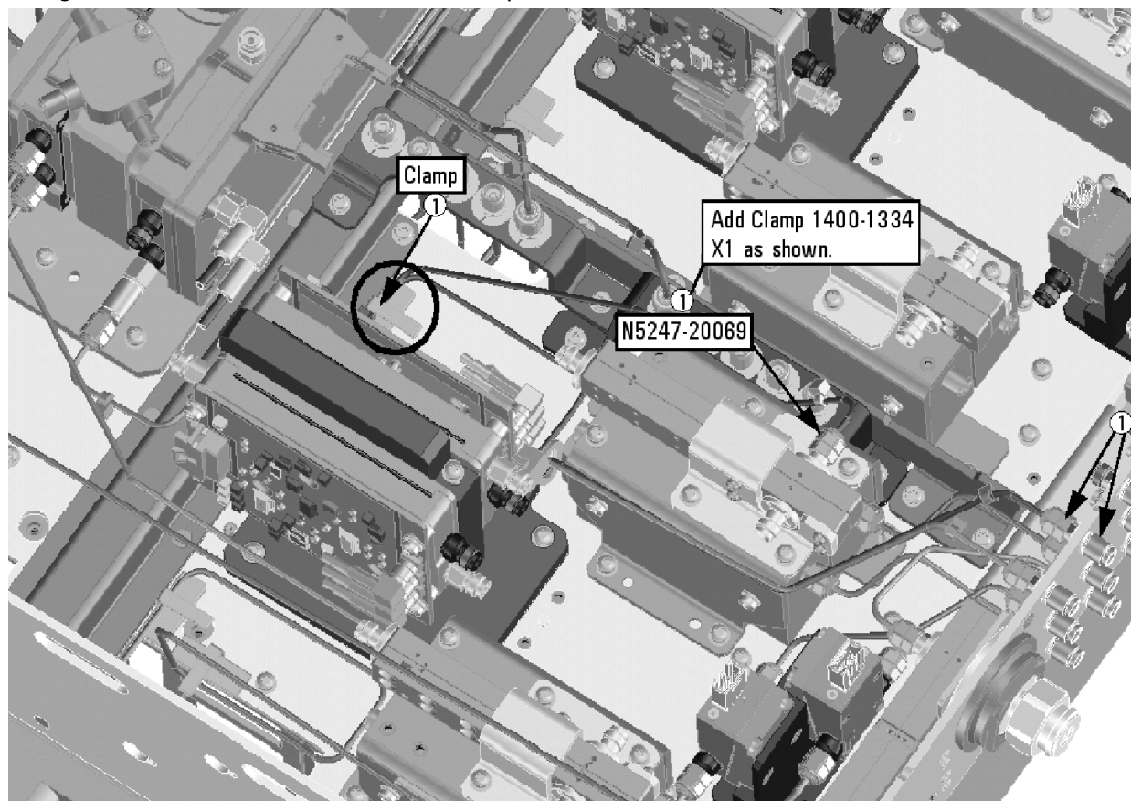
Figure 7-3 Location of Cable Clamp (1400-1334) to Secure W41 (N5247-20069)
