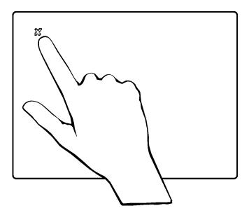
The calibration will time out within 10 seconds if you do not touch the center of the X. You can also press Esc on an optional keyboard to exit the touch screen calibration.
