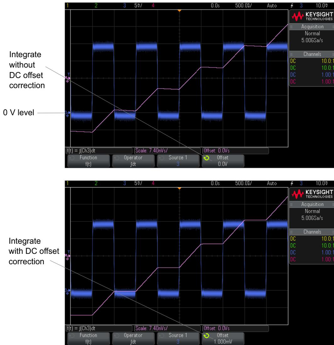
**Figure 8** Integrate and Signal Offset
