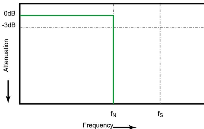
**Figure 34** Theoretical Brick-Wall Frequency Response
