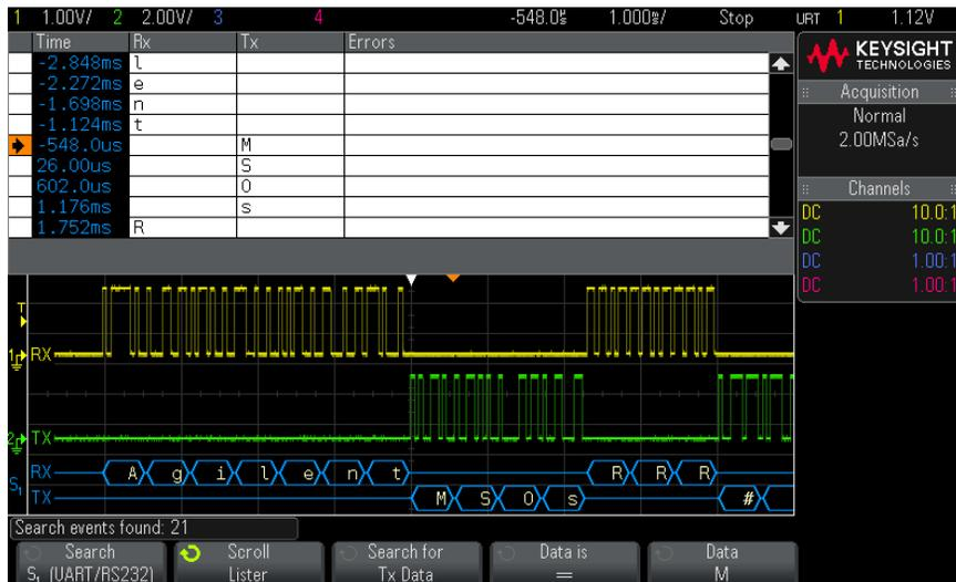
Each serial decode option lets you find protocol-specific headers, data, errors, etc.
