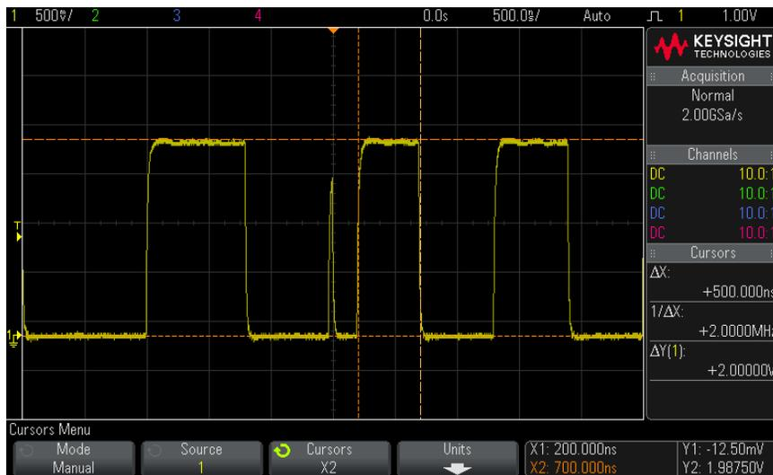
**Figure 43** Measuring pulse width with cursors
