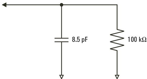
**Figure 21** DC and Low-Frequency Probe Equivalent Circuit
