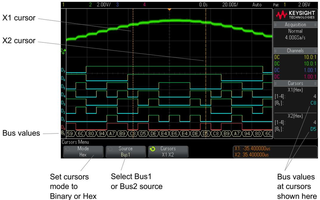
**Bus values are displayed when using Pattern trigger**
