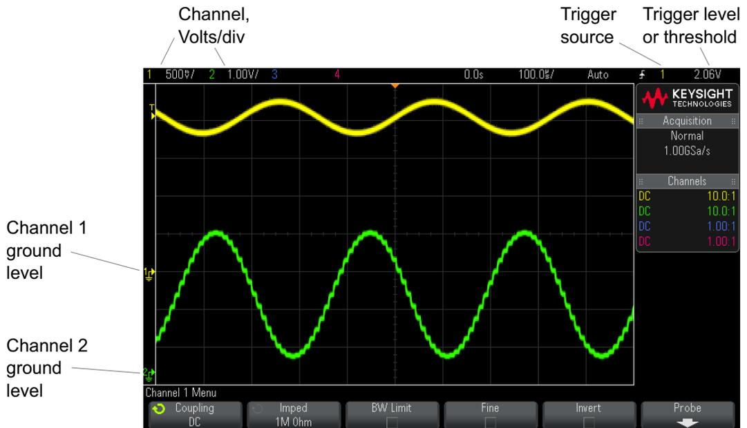
The ground level of the signal for each displayed analog channel is identified by the position of the
