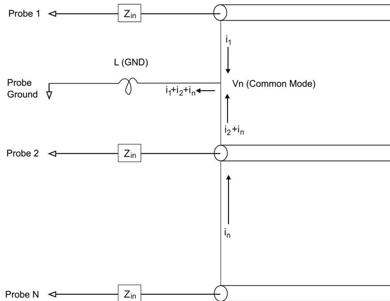
**Figure 24** Common Mode Input Voltage Model
