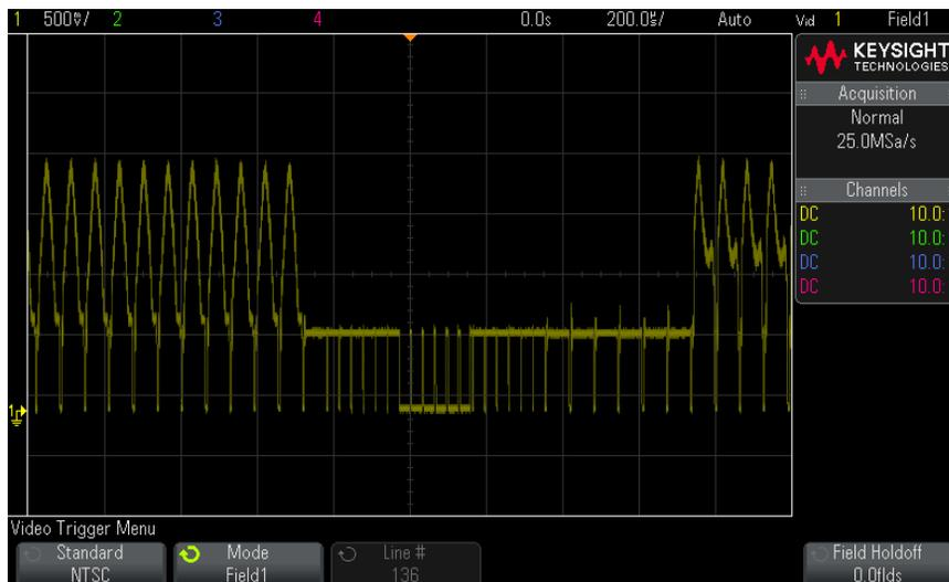
**Figure 29** Triggering on Field 1
