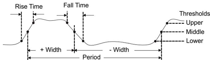
The default lower, middle, and upper measurement thresholds are 10%, 50%, and 90% between Top and Base values. See "**Measurement Thresholds**" on page 234 for other percentage threshold and absolute value threshold settings.
