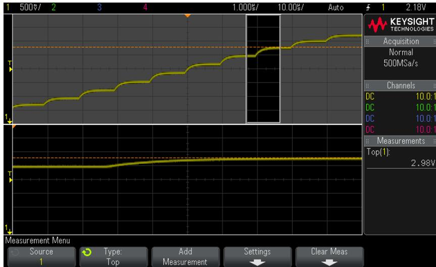
**Figure 46** Isolating area for Top measurement
