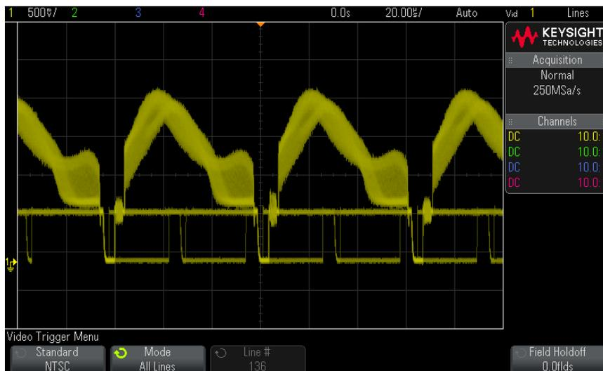
**Figure 28** Triggering on All Lines
