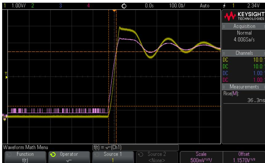
**Figure 10** Example of  $\sqrt{\phantom{x}}$  (Square Root)
