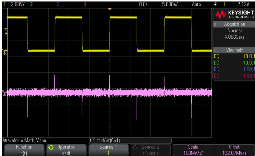
**Figure 7** Example of Differentiate Function
