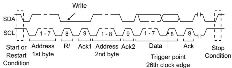
**5** If you have set the oscilloscope to trigger on an EEPROM Data Read condition:
