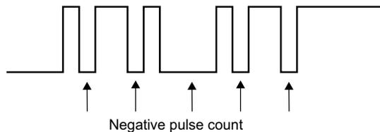
This measurement is available for analog channels.
