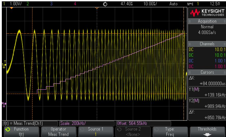
**Figure 17** Example of Measurement Trend
