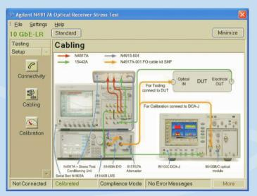
The setup has to be calibrated before any testing can be done.
