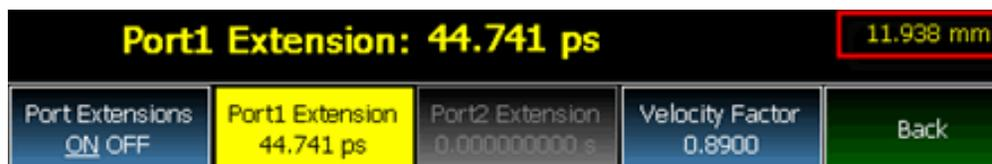
**While setting Port Extension, the physical length of the extension, at the current Velocity Factor setting, is visible to the right (red box in above image).**
