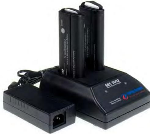
The external battery charger (N9910X-872), lets you charge a fully depleted battery in approximately three hours. It is a two bay, level-3 stand-alone battery charger that is compliant with the standard Smart Battery System. The two bays are charged sequentially on a first-come, first-served basis, though a discharge can be performed in the left bay while the right bay is charging.
