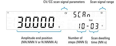
4 After configuring the scan signal parameters, press **Shift** > **Save** to save, and **Shift** > **Exit** to exit the utility menu.
