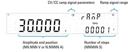
4 After configuring the ramp signal parameters, press **Shift > Save** to save, and **Shift > Exit** to exit the utility menu.
