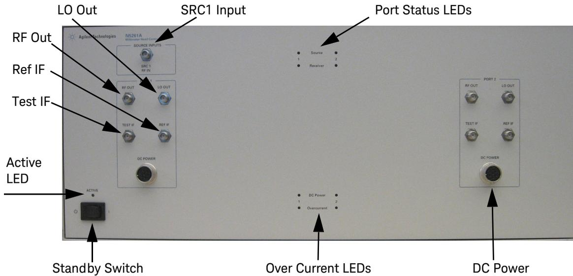
Figure 1-4 N5262A (4-Port) Front Panel Features
