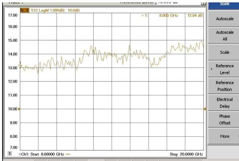
**Figure 2-16** RF Output Gain with +2 dBm ALC Off
