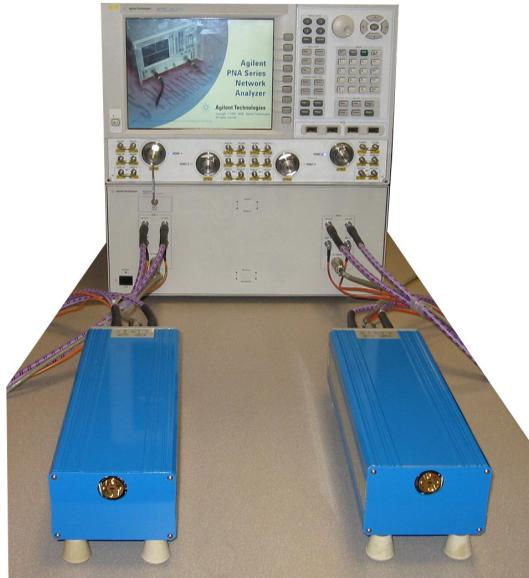
Figure 1-2 4-Port Banded Millimeter-wave Configuration (N5262A)
