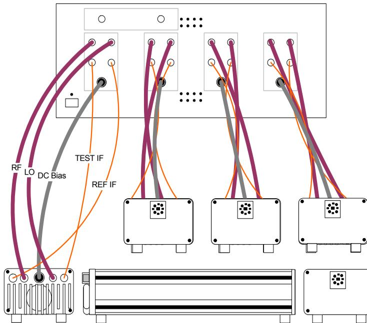
Figure 1-24 Example - VDI Module Connections
