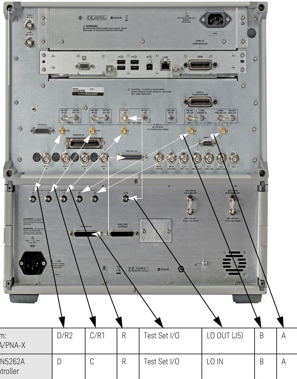
Figure 1-17 N5261A Rear Panel Configuration C
