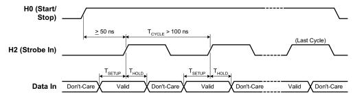
For example, the following SCPI commands set a 34950A in slot 5 to have an 8-bit input using synchronous handshake with an external strobe input. The number of bytes to read into memory is set to infinite (continuous reading into memory until the memory is stopped). The memory is enabled and then triggered. The start/stop line is set high following the first byte handshake and remains high until the last byte is captured.
