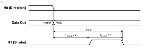
For example, the following SCPI commands set a 34950A in slot 5 to have a 16-bit output using synchronous handshake. Two data outputs are then performed and the strobe line is pulsed for each. The I/O direction line is set low following the first SOURce:DIGital:DATA:WORD command and remains low until the digital channel is reset of reconfigured.
