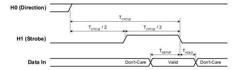
For example, the following SCPI commands set a 34950A in slot 5 to have a 16-bit input using synchronous handshake. Two data inputs are then performed and the strobe line is pulsed for each query. The I/O direction line is set high following the first SENSe:DIGital:DATA:WORD? query and remains high until the digital channel is reset or reconfigured.
