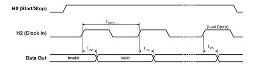
For example, using the *internal* strobe, the following SCPI commands set a 34950A in slot 5 to have a 32-bit output using synchronous handshake. The number of times to output the traces is set to 4. A trace is then loaded into memory and assigned to the channel. The memory is enabled and then triggered. The start/stop line is set high following the first byte handshake and remains high until the last byte is output.
