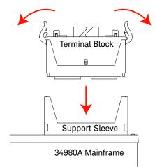
...until the terminal block stops at the two points indicated by the arrows below.
