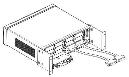
Keysight 34980A (shown with Reverse Rack Mount brackets installed)
