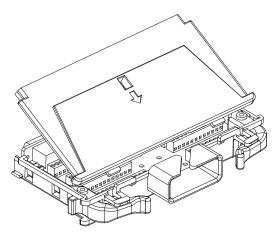
**3** Make connections to the individual terminals as appropriate. Use a suitable wire type, gauge and insulation for your application. Use a 2.5 mm cable tie as shown for additional strain relief.
