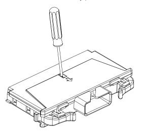
**2** While pushing the tab (Step 1), lift the clear plastic cover from the edge near the D-sub connectors. Slide the cover from under the tab holders and remove the cover.
