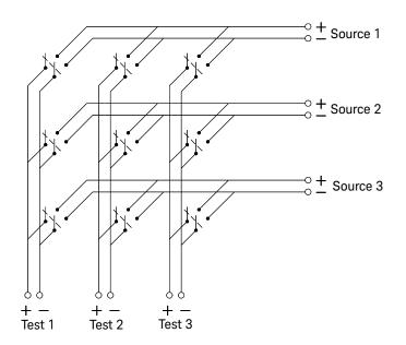
In a matrix switch configuration, any one of the signal sources can be connected to any one of the test inputs. Be aware that with a matrix, it is possible to connect more than one source at the same time. Therefore, it is important to make sure that hazardous or unwanted conditions are not created by these connections.
