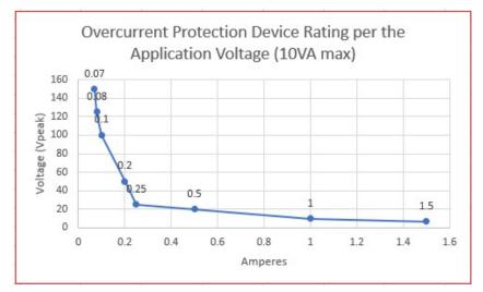
The overcurrent protection devices will be rated, or the snubber circuits will limit the current, according to:
