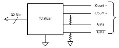
You can configure the totalizer to count on the rising edge or falling edge of the input signal. The minimum rise/fall time for input signals to the totalizer is 5  $\mu$ S.
