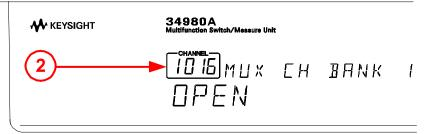
**3** Press **Channel** (*in the Configure key group*) to access the configure menu for Channel 1016. Note that the Channel key lights while in the menu.
