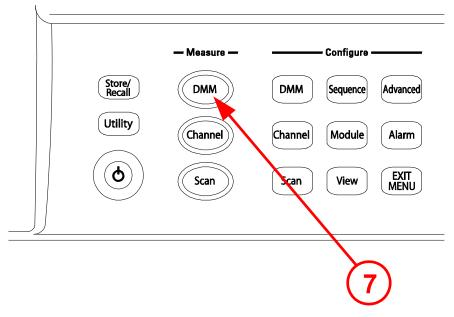
Note that the key lights and continuous ac voltage measurements are made using the internal DMM.
