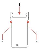
**5** Install the module into a mainframe slot until it fully seats with the backplane connector. Using a Pozidriv #1 screwdriver, tighten the two screws to secure the module in the mainframe. Installation of the support sleeve is now complete.
