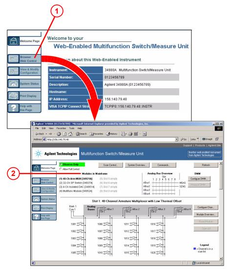
**2** From this page, you can view and modify the configuration of the modules currently installed in the 34980A.
