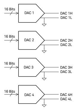
You can set the output voltage to any value between -16 Vdc and +16 Vdc, in 500  $\mu\text{V}$  steps on any or all four channels.
