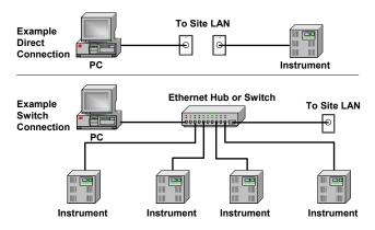
An *Isolated LAN* network is defined as a local area network (LAN) in which computers and LAN-enabled instruments are <u>not</u> connected to a site LAN. Use the crossover cable provided with the 34980A to make a direct connection between the 34980A and your computer. Crossover cables are also supported by many newer LAN switches or routers.
