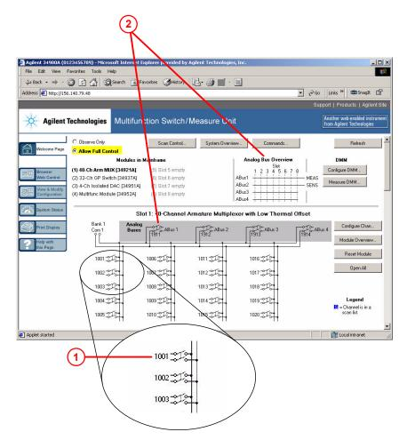
2 You can also open and close the four Analog Bus relays by left-clicking the graphics of these relays. The **Analog Bus Overview** display located near the top of the window shows the slot-by-slot status of the four Analog Buses.
