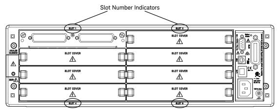
The slot and channel addressing scheme for the 34980A follows the form sccc where s is the mainframe slot number (1 through 8) and ccc is the three-digit channel number. Note that MUX channels numbers are derived differently from matrix modules, and channel numbers for matrix modules are derived differently between 1-wire and 2-wire configuration modes.
