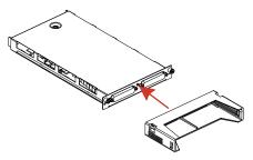
**4** Replace the panhead screw. Then replace and tighten the two flathead screws to secure the sleeve to the module.
