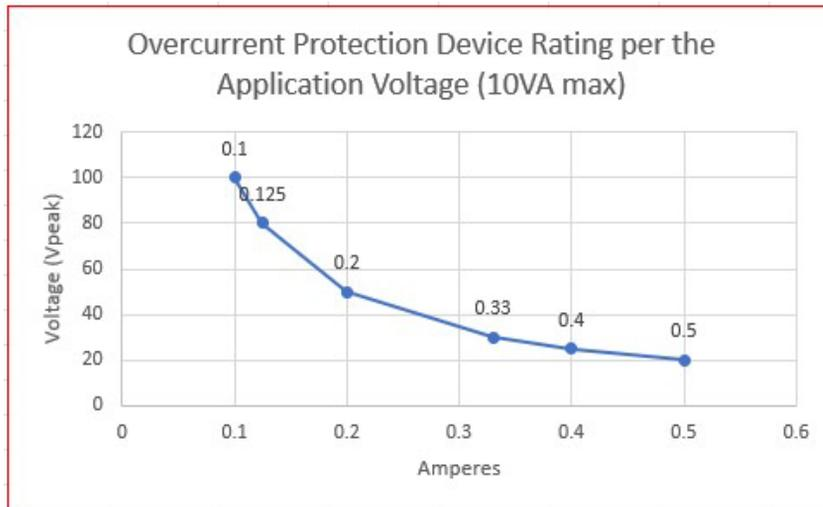
1. Peak voltage, channel-to-channel or channel-to-earth.
