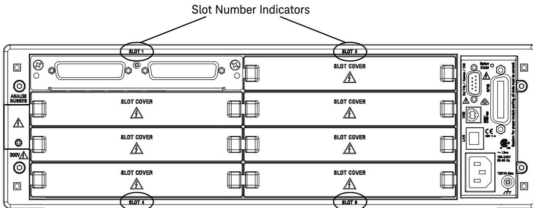
The slot and channel addressing scheme for the 34980A follows the form  $sccc$  where  $s$  is the mainframe slot number (1 through 8) and  $ccc$  is the three-digit channel number. Note that MUX channel numbers are derived differently from matrix modules, and channel numbers for matrix modules are derived differently between 1-wire and 2-wire configuration modes.
