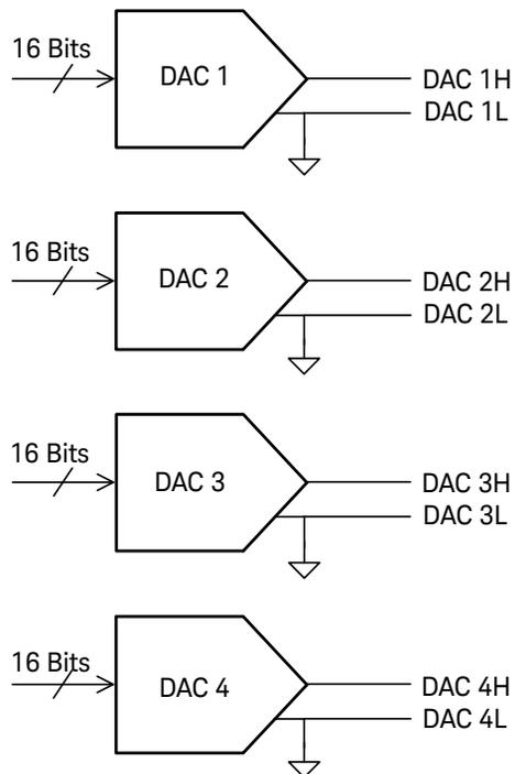
You can set the output voltage to any value between -16 Vdc and +16 Vdc, in 500  $\mu$ V steps on any or all four channels.
