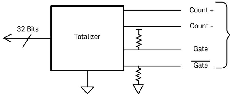
You can configure the totalizer to count on the rising edge or falling edge of the input signal. The minimum rise/fall time for input signals to the totalizer is 5  $\mu\text{S}$ .
