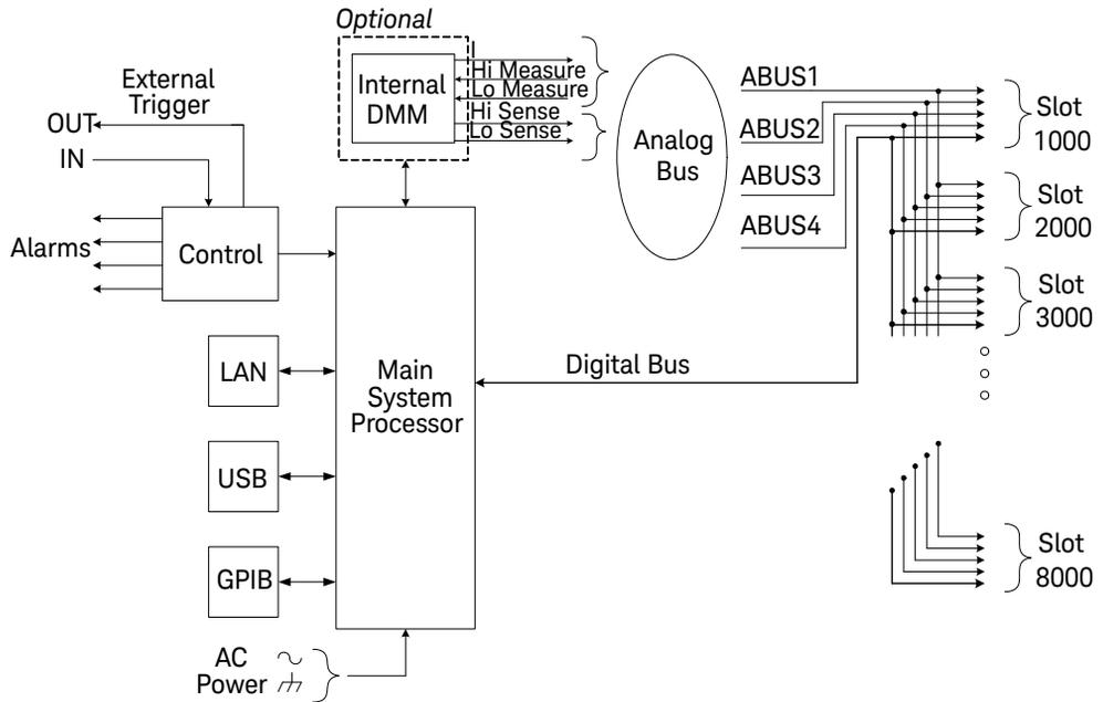
The main system processor also controls activity on the four hardware alarm outputs and external triggering lines. You can use the alarm output lines to trigger external alarm lights, sirens, or send a TTL pulse to your control system.
