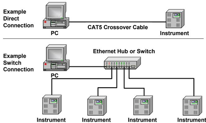
The diagrams above show examples of typical site LAN and isolated LAN networks. Select the LAN network type that you will use to connect the 34980A to your computer. Then follow the corresponding procedures shown on [“Connecting Via Site LAN”](#) on page 90 or [“Connecting Via Isolated \(Non-Site\) LAN”](#) on page 93.
