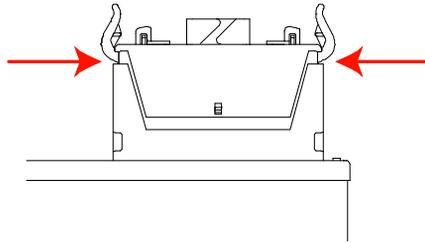
2 Carefully rotate the levers upward as shown...
