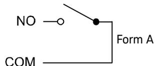
Form C switches are also called Single-Pole, Double-Throw (SPDT) and contain a normally-open (NO) and a normally-closed (NC) contact. Form A switches are also called Single-Pole, Single-Throw (SPST) and contain a normally open (NO) contact, which is either open or closed.
