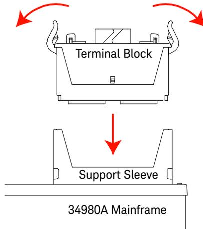
...until the terminal block stops at the two points indicated by the arrows below.
