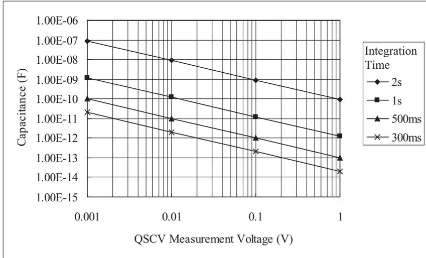
**Figure 9-2** Maximum Measurement Value Using 1 nA Range: HPSMU, MPSMU, HRSMU, ASU+SMU
