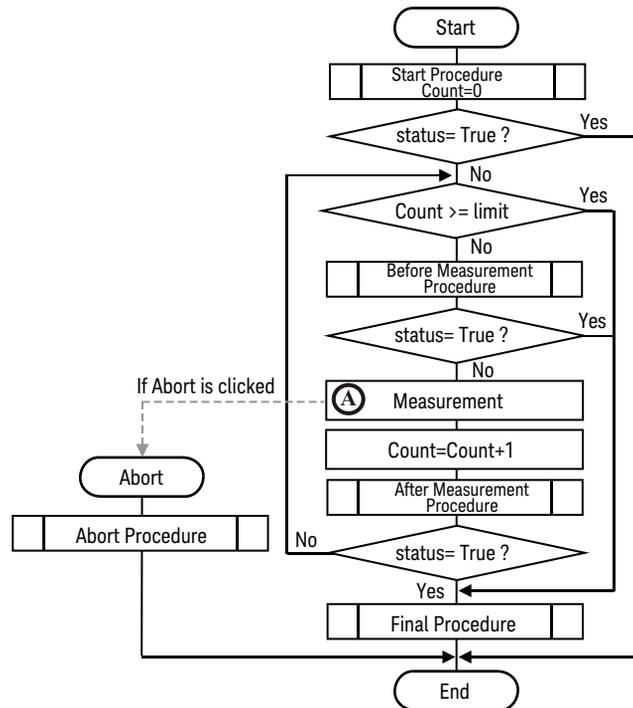
The repeat measurement is performed as shown in this flowchart. The status is a response returned by each procedure. The Count is the accumulated number of test executions. They are the stop condition of the repeat measurement.
