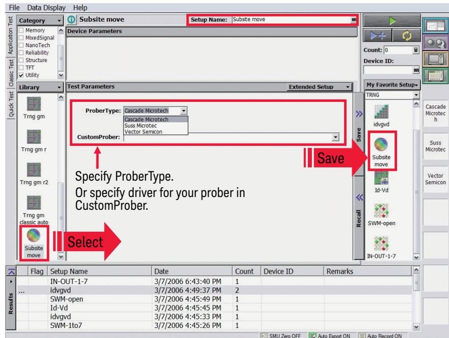
The Subsite move setup moves wafer chuck to the next subsite, reads device ID from the prober, and sets it to the Device ID of the test result record.
