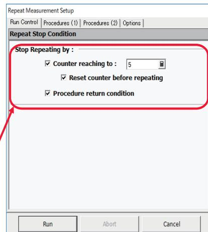
The procedure is called after one of the stop condition is detected. This procedure sets wafer chuck to the DOWN position.
