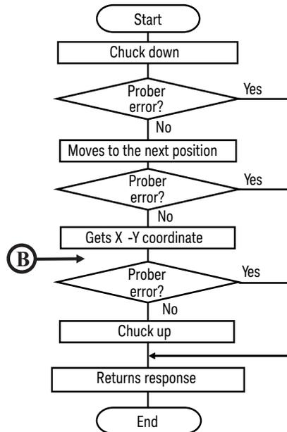
The procedure is called after the measurement is completed for a die. This procedure sets wafer chuck to the DOWN position, moves it to the next probing position, checks the prober status, gets the X-Y coordinate of the probing position, and sets the wafer chuck to the UP position. At last, the procedure returns the response.
