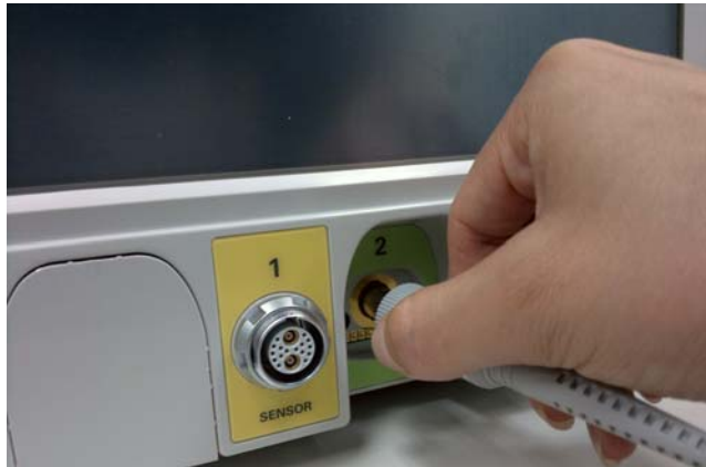
Figure 1-12 Connecting the probe to the 8990B
