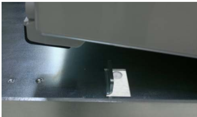
Figure 1-21 Raised tabs in the support tray
