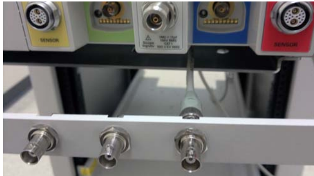
Figure 1-27 Connect the BNC connector to the bottom trim plate
