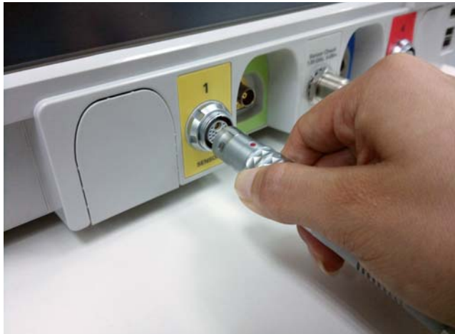
Figure 1-11 Connecting the sensor cable to the 8990B
