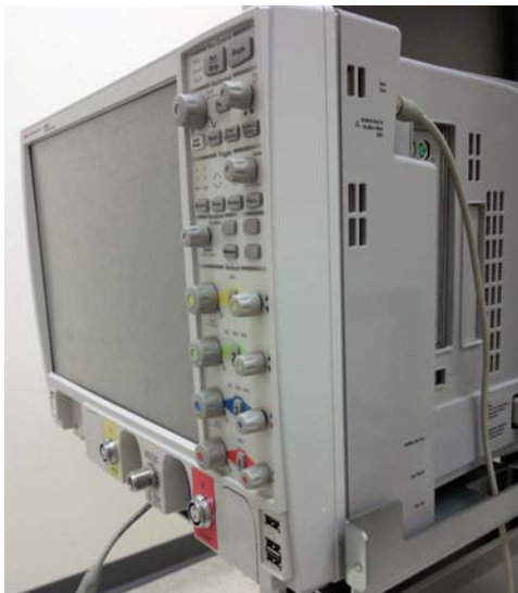
Figure 1-23 BNC connectors to the rear of the 8990B
