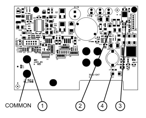
Figure 5-2. Bias Board Test Points
