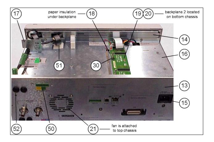
Figure 6-2. Top Cover Removed
