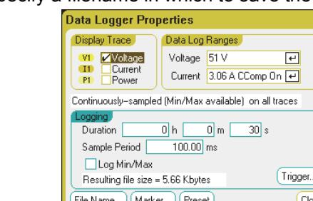
**2. Press **On** to turn on the data logger**
