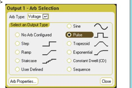
**4. Press **Properties**. Use the navigation and number keys to configure the Pulse properties.**
