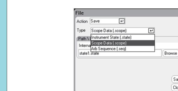
**3. Navigate to the File Name field and enter the name under which to save the scope data.**
