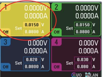
**2. Press the Select Output keys, or use the navigation keys to select a different output.**
