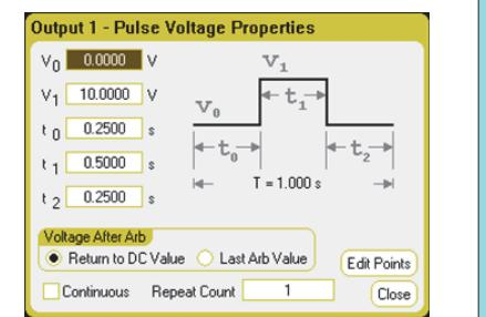
**5. Press **Close** or **Back**. Use the navigation keys to select the trigger source for the Arb.**
