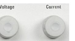
The front panel V and A Set fields will indicate the values that the voltage and current are set to. Watch the values change as you rotate the knobs.
