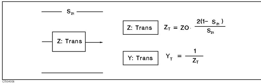
**Figure 4-3. Z:Transmission Model**
