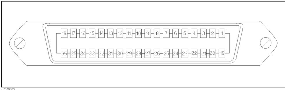
**Figure 8-13. Parallel I/O Port Connector Pin Numbers**
