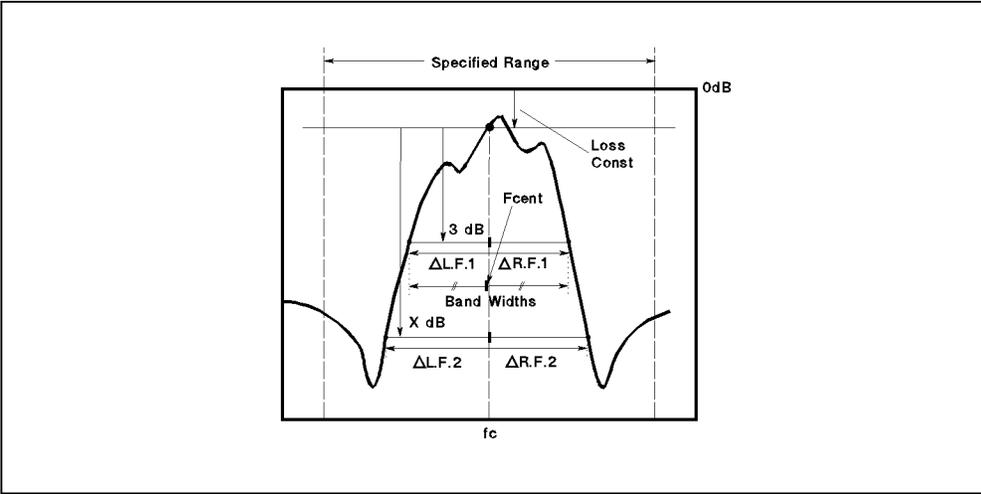
Figure 6-4. Filter Parameter for  $-3\text{ dB BAND WIDTH}(F_c)$
