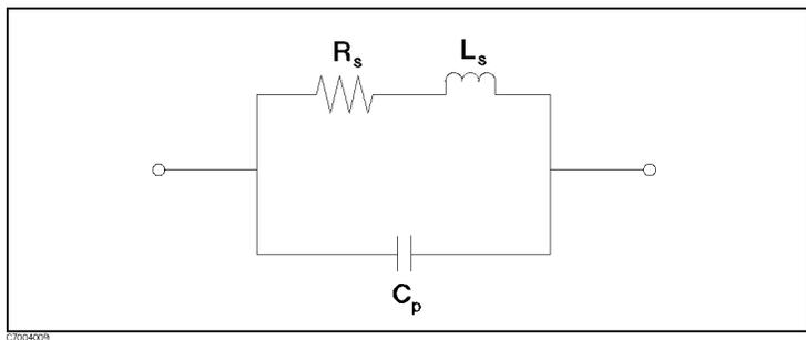
**Figure C-1. Equivalent circuit model of calibration standard**
