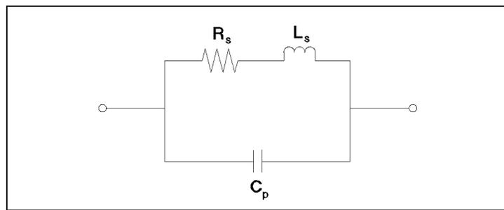
Figure 4-8. Equivalent Circuit Model of Standards
