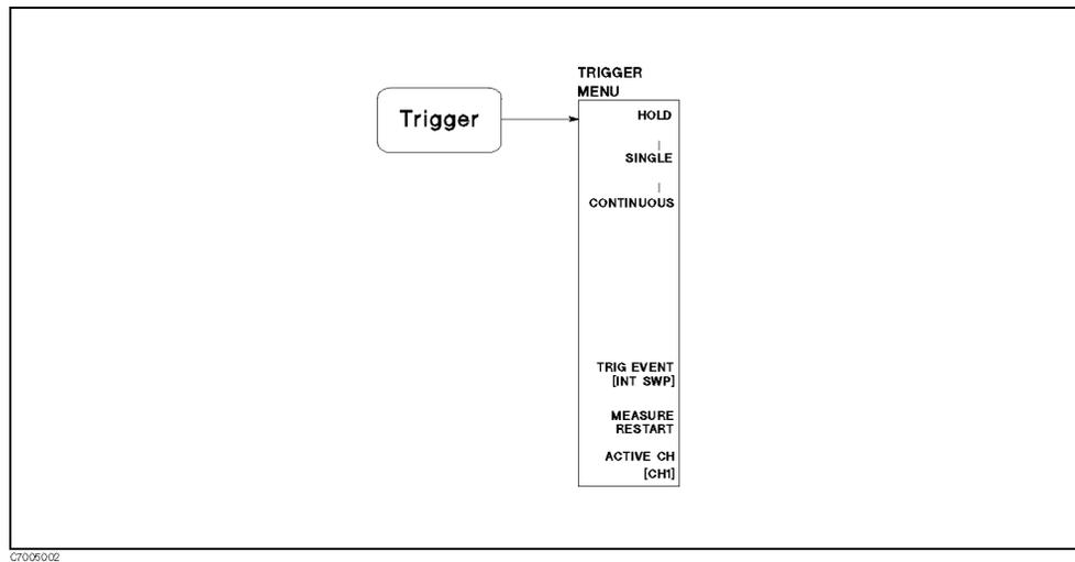
Figure 5-2. Softkey Menus Accessed from the **Trigger** Key
