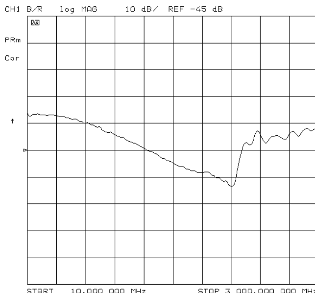
Figure 2-35 Example Mixer LO to RF Isolation Measurement
