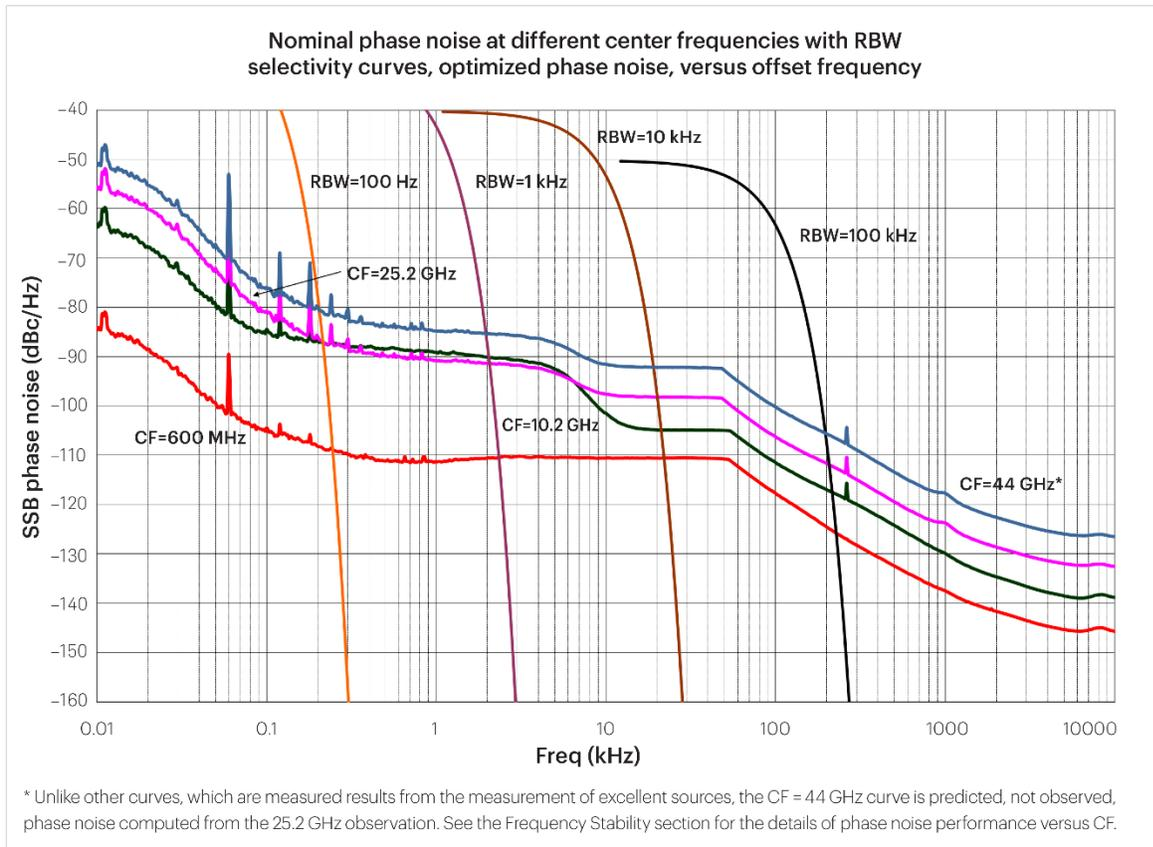
**Figure 1.** Nominal phase noise at different center frequencies
